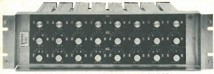
The Altec Lansing 24-filter Acousta-Voice equalizer. Each of the filters can be adjusted in 1-dB steps.
