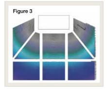
VARIA's flexibility in coverage patterns enabled a design where all arrays can line up precisely to each major seating section, creating strong acoustical cues to the stage (**Figure 3**). The arrays were designed strictly around angular coverage requirements.
