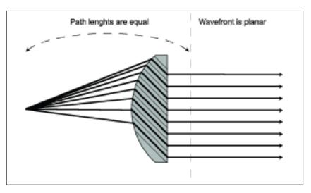
Figure 4: The path length refractor can generate planar wavefronts over a wide operating band.
