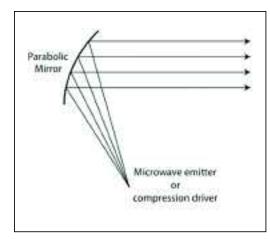
Figure 1: Whether for microwaves or sound, reflectors operate on a "ray" model.
