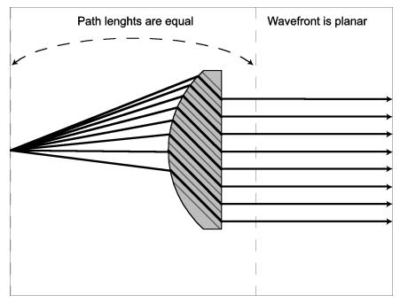
But what happens at lower frequencies, when the "wave model" takes over due to the longer wavelengths? The path length refractor lens then functions as a closely spaced array of diffraction slots, as illustrated below:
