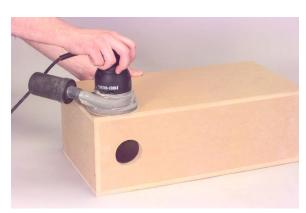
2. Clean and dry the cabinet. Make sure to remove any and all dust from the surface. Any loose dust may cause dimples and will decrease the effectiveness of the adhesive.
