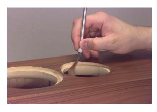
13. Going over the edges of MDF with a marker that matches your vinyl will help minimize the visibility of any gaps between the driver and the vinyl.
