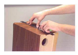
10. Remove the excess material from either side of the seam and gently press the vinyl back into place. The result should be a perfect butt joint in the covering.
