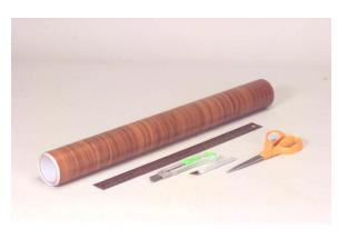
4. Cut the vinyl laminate to rough dimensions of your box size, leaving 1-2 inches extra in all dimensions. For quickest installation, a single piece of laminate may be used to wrap completely around the sides and top of the cabinet. This will provide seamless corners and a single seam on the bottom of the cabinet. **Hint:** Follow the grid on the rear of the vinyl to ensure straight edges, which will help in aligning grain and keeping application straight.
