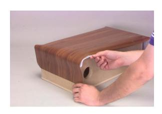
6. When the corners of the cabinets are reached, be sure to pull the veneer very tight as you proceed. A loose corner will end up with air bubbles or a wavy look. **Hint:** If you have an extra person available it would be helpful to have them press the vinyl down as the veneer is stretched around the corner. Also note that it is much easier to work with the vinyl if the unused portion is kept rolled up.
