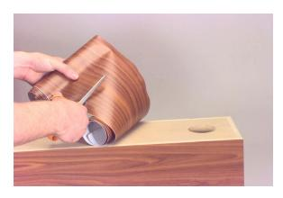
11. After the vinyl is pressed into place, trim edges using the same method as previously used. As long as the blade is held perpendicular to the workpiece, the blade should not damage the existing vinyl. **Hint:** A thin piece of tape may be placed on the side panels to prevent damage, though it will likely be found that this is not necessary.
