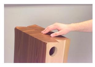
9. Trim the excess material off of the sides at the front and back using a very sharp razor knife. Be sure to hold the blade perpendicular to the front as you cut, which will ensure a straight seam. **Hint:** Holding the trimmings at the appropriate angle and tension will allow a very smooth and easy cut.
