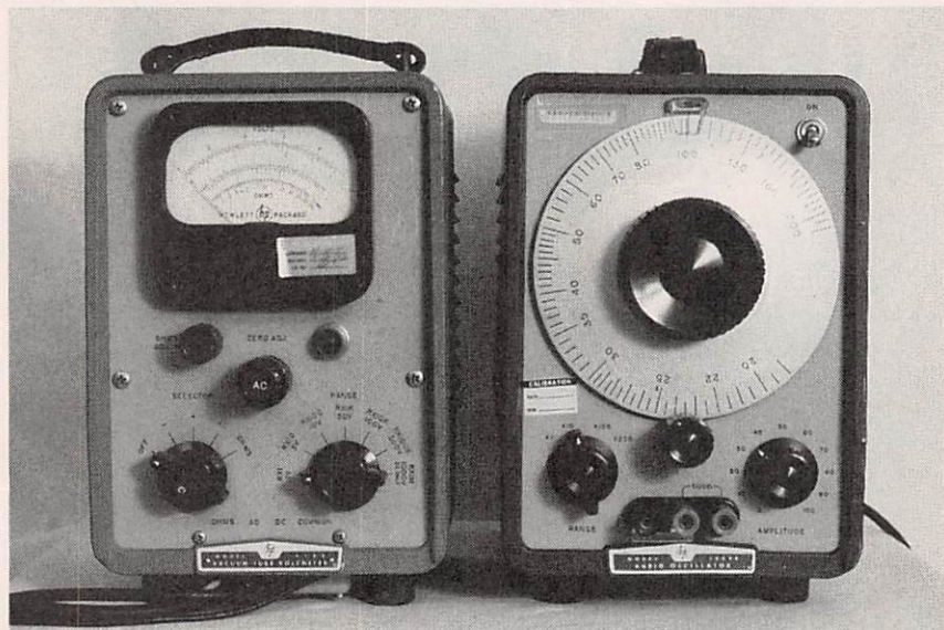
Fig. 3. Two examples of vintage vacuum-tube test equipment from Hewlett Packard: a Model 410 VTVM (left) and a Model 200 audio oscillator.
