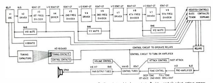
Oscillator ond dividers provide tones over 6-octave range. Oscillator is tuned by key contacts. Register controls select octave ranges.
