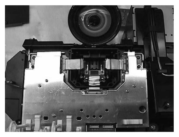
Now carefully lift the brown tabs that hold the ribbon cables in place. With the brown tabs in the up position remove the ribbon cables by slowly pulling them straight out. See picture below before attempting.
