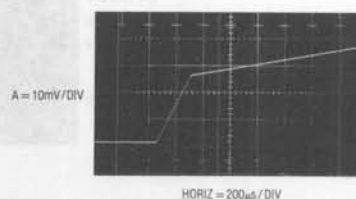
Figure 13. Detail of the Switched Slope Capacitor Charging
