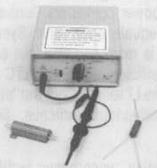
Figure C3. Typical Current Shunts and an "Isolated" Probe
