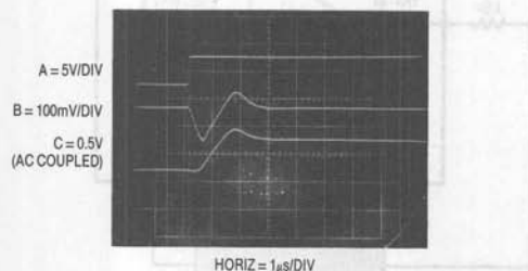
Figure 4. Transient Response for a Full Load Step. Follower Connection Provides Clean Dynamics.
