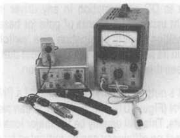
Figure C1. Various Current Probe Types Provide Different Capabilities. Selection Criteria is Application Dependent.
