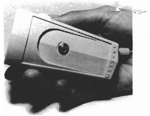
THE HAND-HELD IR FINDER. Pointing it at heat raises the note in the earphone.
