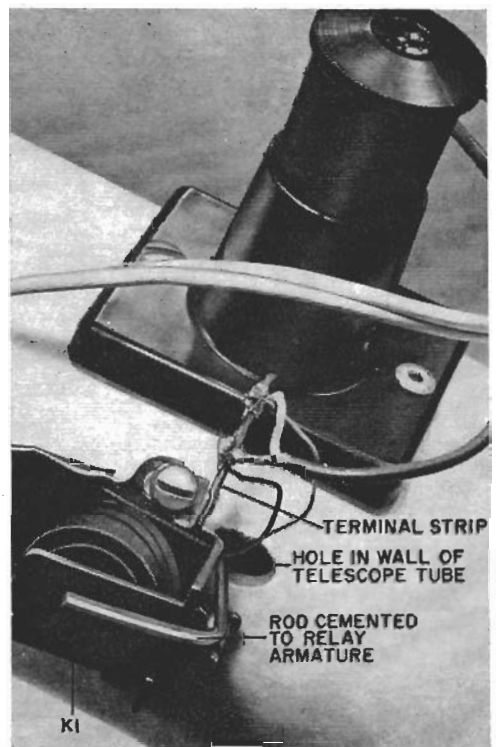
The transmit-receive relay is mounted to the telescope tube with the solar cell and rod passed inside through a hole cut in the telescope tube wall.
