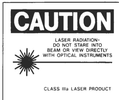
FIG. 8—ANY LASER DEVICE must contain warning labels according to the specific type of device. Our hand-held laser must display this warning, in addition to a label stating that it conforms to specifications and a warning at the laser aperture.
