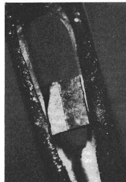
FIG. 4—THIS SEMICONDUCTOR LASER is so tiny that it can fit in the eye of an ordinary sewing needle. Photo courtesy of ATT Bell Laboratories.
