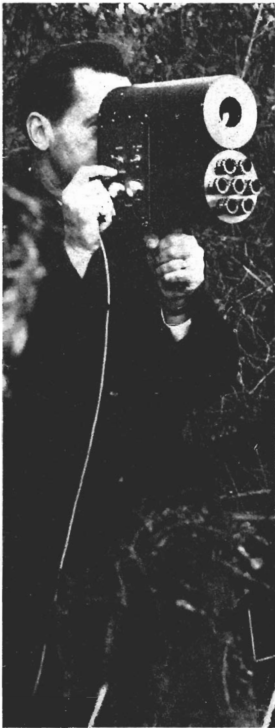
This detection system uses a gallium-arsenide pulsed laser and an image converter viewing tube to find targets up to 300 feet away in complete darkness. Developed by Laser Diode Laboratories.
