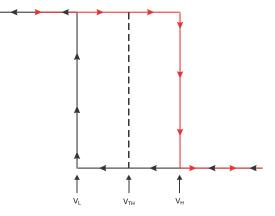
4. Derive the equation for V<sub>H</sub>, which is the threshold voltage when V<sub>o</sub> is high. For simplicity, assume V<sub>o</sub> switches to V<sub>cc</sub> when V<sub>i</sub> < V<sub>L</sub>. When this occurs, R<sub>1</sub> and R<sub>3</sub> are in parallel.
