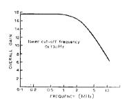
base configuration offers advantages such as small non-linearity of its transfer characteristic and relatively constant gain with frequency, while providing moderate gain due to the impedance transformation between input and output.
