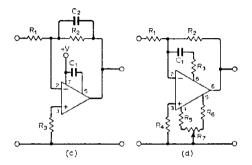
R<sub>1</sub>, R<sub>2</sub>:  $10k\Omega$ , R<sub>3</sub>:  $5k\Omega$ C<sub>1</sub>:  $0.1\mu$ F, C<sub>2</sub>: 5pFShortens settling time to  $1\mu$ s for 0.1% accuracy after 10V step  $R_1$ ,  $R_2$ :  $4.7k\Omega$   $R_3$ :  $3.3k\Omega$ ,  $R_4$ :  $1k\Omega$   $R_5$ ,  $R_6$ :  $27k\Omega$ ,  $R_7$ :  $2.5k\Omega$ Slew rate:  $150V/\mu s$
