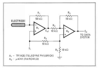
**Plasma probe.** Rocketsonde studies of density and temperature of electrons in the ionosphere may be achieved by measuring the current drawn to an electrode that projects out and is well insulated from the rocket body. The circuit shown here applies potential to the electrode through an op amp, thus avoiding voltage-supply-insulation problems and leakage errors in current measurement. Circuit measures currents from  $10^{-3}$  amperes down to  $5 \times 10^{-11}$  A.
