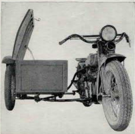
Standard Express Body—Hinged Lid. The carrying space is 45' long, 23' wide and 18' high. Plenty of room between machine and van body for driver's comfort.
