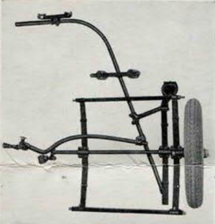
The simplicity and sturdiness of the new Excelsior-Goulding Commercial Chassis is very evident. The wheel is spring-suspended and the body weight is carried on long semi-elliptical springs with two helical stabilizing springs in the front.
