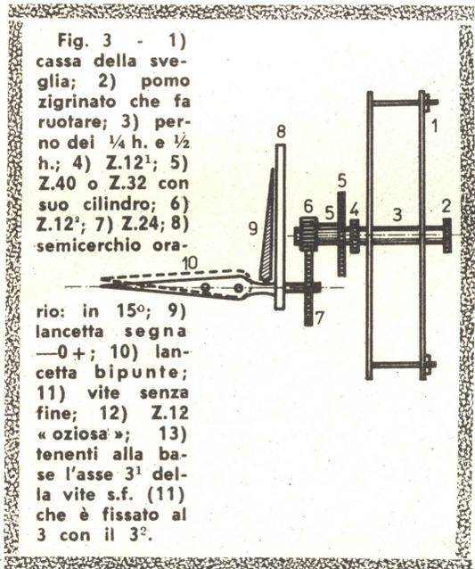
$$\frac{Z.12 \times Z.10}{Z.36 \times Z.40} = \frac{N.120}{N.1440} = \frac{N.12}{N.1} \text{ in } 12h.$$
