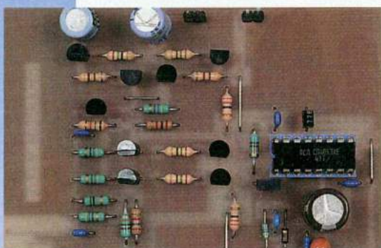
■ Figure 6 : le circuit simple face.
