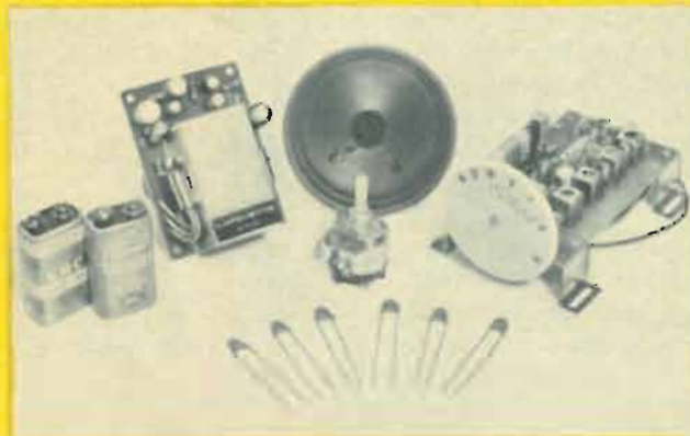
Parts for aviation receiver cost about $20. Author used an AM tuner (right) and a modular 3-watt amplifier for his unit.
