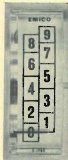
PC module is small (1"x2"x4") and mounts all readout components: decade counter, decoder/driver, and modified panel meter.
