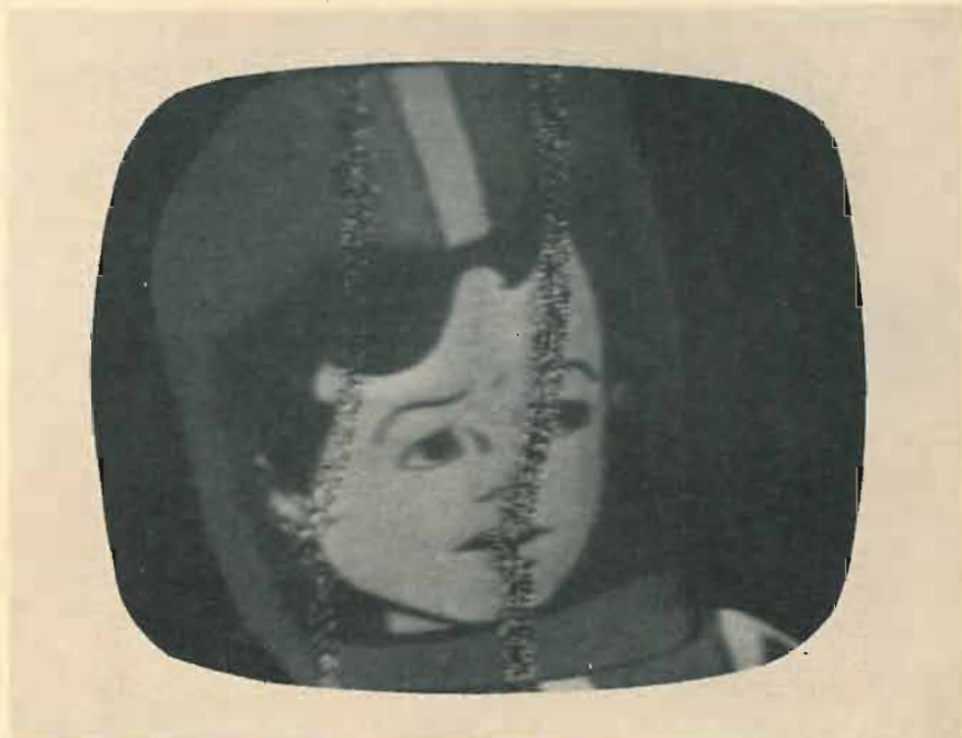
The set had what looked like the worst case of Barkhausen oscillation I'd seen.
