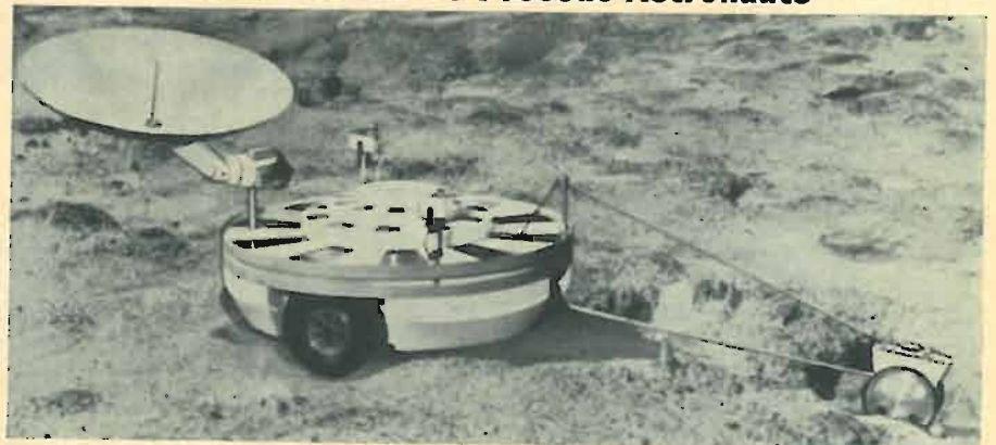
The odd-shaped vehicle is an exploration vehicle, designed by the Westinghouse Defense Center to make the arrival of astronauts on the moon safer, and to make the work more useful. It would arrive before the astronauts and roam the surface of the moon to locate landing sites for manned vehicles. Stereo television cameras would scan the moon's surface and transmit images back to earth. The little wheel ahead of the vehicle detects crevices, and is also designed to collect samples of the surface for analysis.
