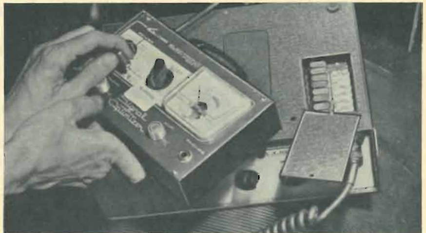
Most CB transceiver trouble is caused by bad tubes or bad crystals. This Globe device doubles as power output meter and crystal checker.
