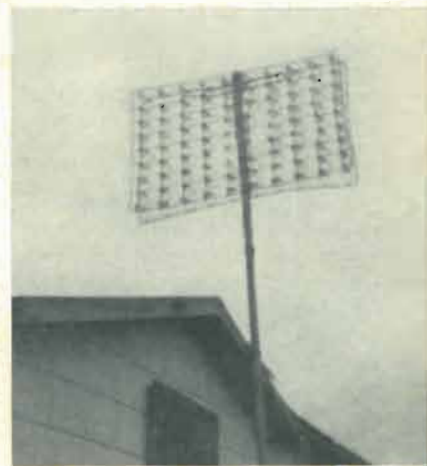
The multi-helical array looks more like a search radar antenna than an ordinary gatherer of TV signals.
