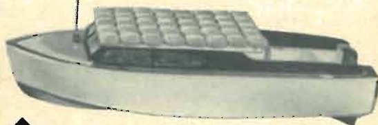
▲ SOLAR-POWERED BOAT uses 40 solar cells to run its small motor, moving majestically through the water under radio control on sunny days. The sun ship was built by the Rev. Robert W. L. Mark of Hawley, Pa., known to RADIO-ELECTRONICS readers as author of articles on the old one-tube Twinplex circuit.
