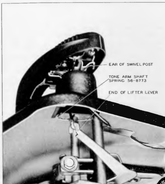
Figure 2. Tone-Arm Height and Lift Adjustments and Vertical Timing Adjustments
