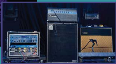
Guitar/bassist Dapose's setup includes a Vox AC30 for guitar and an Ampeg 400W classic tube head with 4x10 Ampeg cabinet for bass. Worthington miks the guitar with a Beyer M68 cardioid dynamic, while bass takes a Sennheiser 604 hung with a homemade spatula/z-bar. "I also take the direct out from his bass amp," he says. "Dapose keeps his signals separate—guitar through the guitar amp and bass through the bass amp—resulting in fewer blown guitar speakers!"
