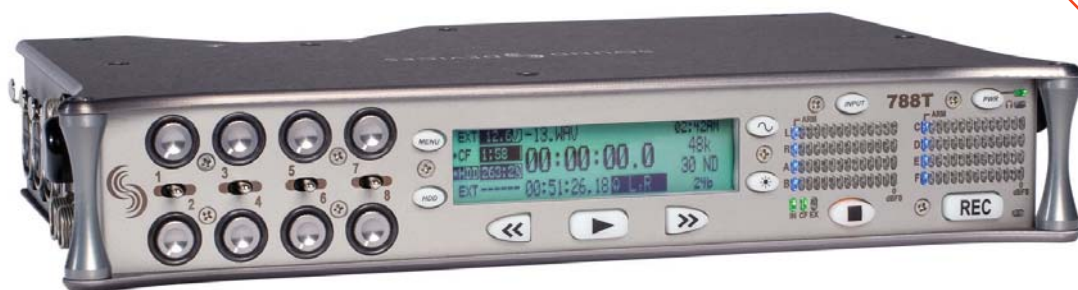
The 788T's front panel features 112-segment (8x14-inch) sunlight-viewable meters, gain control and a backlit LCD screen offering a variety of system information.
