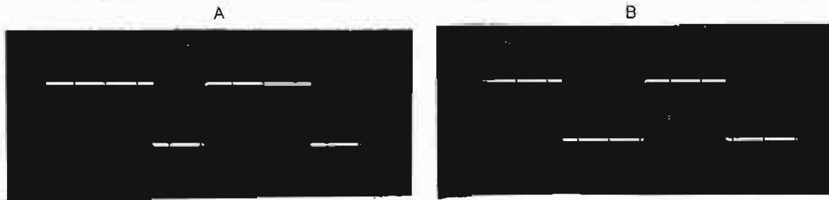
Figure 5: Oscilloscope traces showing relationship of R_a , R_b and the output waveform. At A, R_a = R_b and the output is high twice as long as it is low. At B, R_a = 0 and the high pulse is the same length as the low pulse.
