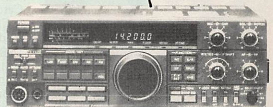
TS 440 SP SSB-AM-FM-RTTY 100 KHz-30 MHz-100 W HF
