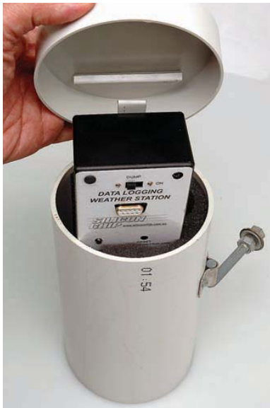
Left: the controller box inside its PVC pipe case. It hangs free on brackets fixed as shown above. The pipe mounting bolt is flexible to allow the pipe to be moved at will.
