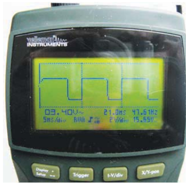
Fig. 11.2. Waveform produced by the astable
