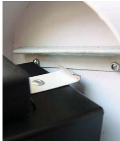
Left: the controller box inside its PVC pipe case. It hangs free on brackets fixed as shown above. The pipe mounting bolt is flexible to allow the pipe to be moved at will.
