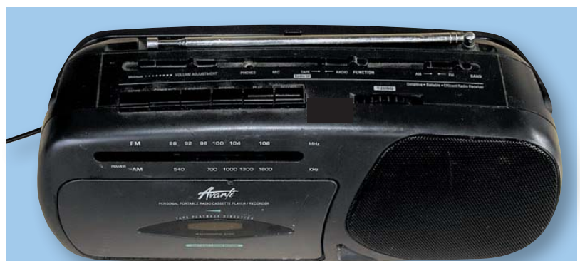
This is the cassette player that donated its amplifier. In many cases it will be easiest to use the original cassette player power supply and mount the new components inside.
