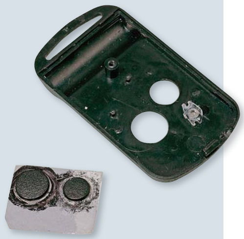
Above: the finished transmitter board inside its keyfob-style plastic case. Power comes from a 12V A23 car alarm battery. Note how the keyswitch covers are mounted on the lid, using a 20 × 24mm silicone washer – see text.
