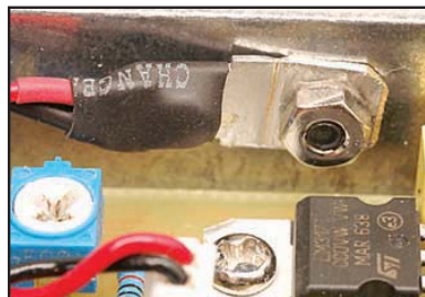
Here's how the thermistor (TH2) is 'heatshrinked' to a spade lug and then secured to the box side.
