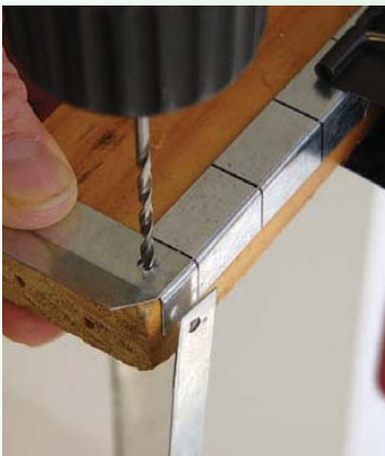
Drilling holes in small, thin bits of metal is not only tricky, it can be dangerous if you don't properly clamp and support the work.
