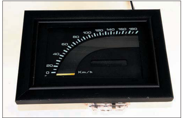
The speedo was mounted in a small picture frame. Note that it is easy to backlight the dial – all car speedos have this facility, and in some, even the needle is illuminated!
