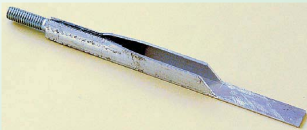
The mounting bar is made from a piece of U-shaped (channel) aluminium with an 8mm bolt crushed in position then secured with two-part epoxy. This is then secured to the (inner) top cover with pop rivets. The outer top cover, which helps prevent the housing from heating up and giving false readings, is mounted 12mm above the inner top cover by means of 12mm threaded nylon standoffs so there is no heat conduction from one part to the other.
