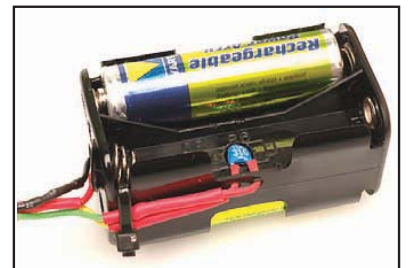
The battery temperature thermistor (TH1) is mounted inside a modified battery holder so it contacts two cells.
