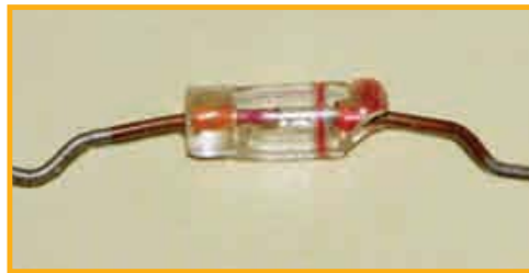
Fig.2. If a diode looks as though it is tiny, fragile and in a glass encapsulation, then it probably is. Any flexing of a lead near the casing can result in damage, as in this example
