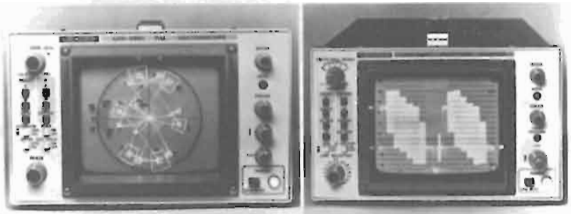
Fig. 2 - LVS 5851 e LBO 5861, Video-Signal Instruments LEADER.
