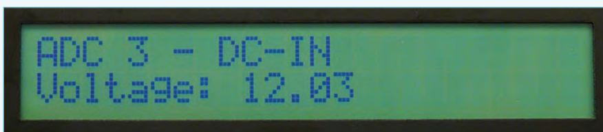
Figure 8. Channel 3 measures the supply voltage to the circuit (12 V nominal).
