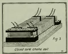
A Well-Designed Choke Coll of the Double-Pole, Closed-Core Type. One-half of the Winding is Placed on Each Leg of the Lami-nated Sheet Iron Core.
