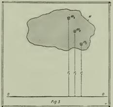
Fig. 3. Another Form of Expression for the Energy of a Rotating Body May Be Obtained by Determining Its Moment of Inertia. Here the Mass M is Subdivided Into Minute Parts m<sub>1</sub>, m<sub>2</sub>, m<sub>3</sub>, ... etc. The Sum of the Products of These Masses and the Squares of Their Distances is the Moment of Inertia, Which with the Angular Speed, Gives the Kinetic Energy E.
