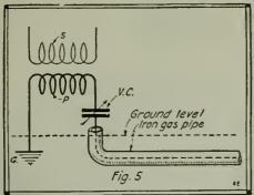
Ground Aërlal Burled in a Continuous Section of Iron Pipe. Excellent Results Have Been Obtained with This Scheme.
