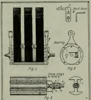
Every Telephone Magneto Can Be Made Over, with Slight Changes, into a First-Rate "Direct-Current" Dynamo. Fine for Auto or Boat Lighting and Experimental Work.
