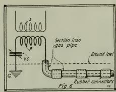
Here the Iron Pipe Jacket Surrounding the Buried Aërial is Divided up into 20-Foot Sec-tions by Means of Rubber-Hose Connectors; a Later Development.
