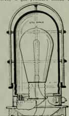
chamber normally maintains the light, but if fumes are present on the outside, this external pressure will cause the light to be extinguished. It operates on the principle that the internal pressure of the gas will normally maintain the light, but should the gas pressure in the chamber he brought to an inferior or superior pressure to that without the chamber, then the light will be extinguished.
