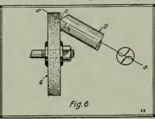
in Grinding or Sharpening Twist Drills by Hand, Care Should Be Exercised to Keep the Drill Axis At An Angle of 60 Degrees with the Grinding Plane.
