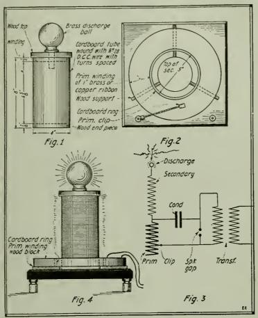
An 8- to 10-Inch Spark Oudin High Frequency Coil. It Can Be Excited by a One-quarter K. W. Step-up Radio Transformer or 6- to 8-Inch Spark Coil.
