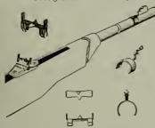
The sighting plate mounted on the front end of the firearm is coated with a covering of luminous paint, or some such other light-radiating pigment, which can be easily discerned at night. The benefit of this improvement in sights is that the marksman looking thru his rear sight can easily discern his forward point or sight due to the fact that the same is covered with this radium paint.
