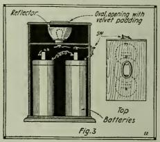
Battery Type of Egg Candling or Testing Cabinet Which Anyone Handy with Tools Can Easily Construct. The Lamp and Re-flector Can be Obtained at Any Supply Store.
