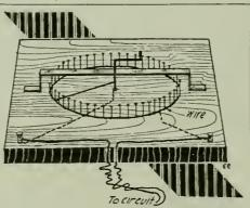
Simplest Circuit Interrupter Formed of a Ring of Nalls, Against Which a Brass Spring Mounted on a Crank Is Turned.
