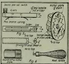
Details of Medical Coil: Handles, Sponge, Electrode and Bipolar Switch.
