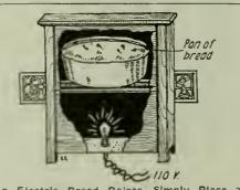
An Electric Bread Raiser—Simply Place a 32 C. P. incandescent Lamp Under the Pan of Bread and Watch the Results.
