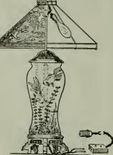
may he formed in one piece with the bowl or may be separate and cemented together in order to pre-vent leakage. The hottom of the bowl is arranged to present a pleas-ing appearance with a hed of sand.
