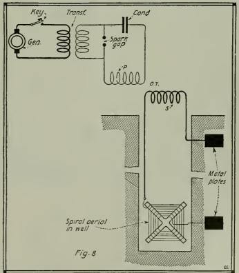
Long wave lengths are tunable by using large condensers and loose "Transmitting with the Rogers Underground Aërial. In This couplers preferably.
