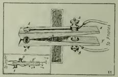
A Handy, Simple and Efficient 'Phone Con-necting Clip. The Clip Is Clamped, on a Strip of Fiber, Lined on Elther Side with Brass Strips as Shown.
