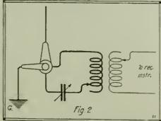
Using One Buried Aërial and Earth Gives Same "Directivity" as When Two Wires Are Used.
