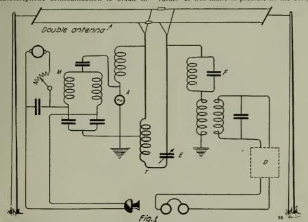
System of Duplex Radiotelephony with Inductive Neutralization Described by Mr. Alexanderson Before the Institute of Radio Engineers. M—Magnetic Amplifier; A—Alternator; T—Neutralization Transformer; E—Exposure Condenser; F—Frequency Trap; D—Detector.
