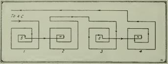
Proper Connection of Poles Composing Starting Winding of Induction Motor
