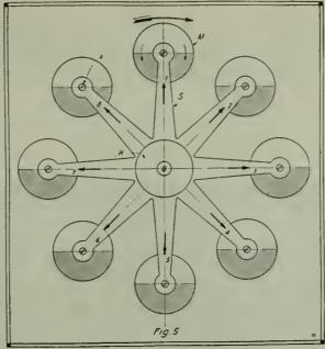
Fig. 5. This Diagram Represents a System Composed of 8 Balls M, Carried on Spokes S, and Rotating Around Center O. The Balls Are Freely Rotatable on Pivots Which Can Be Tightened. With This Model the Fallacy of the Moon's Rotation on Its Axis Is Demonstrable.
