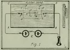
Here. ABCD = Piece of Soft Wood 5 x 3 x ½ Inches Resting on Wooden Base. abcd = Wooden "Mouthpiece" Hanging on Back of Larger Piece and Carrying a Short Carbon Rod. ef. HK and LM = Carbon Rods Attached to the Larger Piece of Wood. Wires Lead from HK and LM Thru the Posts p and q and Two Dry Cells at R to the Standard 75 Ohm Telephone Receiver.
