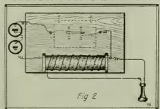
Transmitter Showing Small Induction Coll Mounted on the Front of the Board. The "Mouthplece" Is in Series with the Primary Winding.
