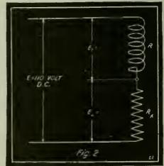
Experiment with Choke Coll Designed for A. C. Circuit Connected to D. C. Circuit, Showing the Effect of Inductance or Impedance on the Current Consumed.
