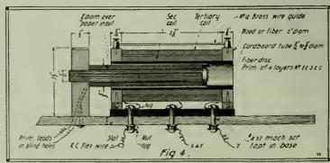
Section Thru the Induction Coll, Provided with Primary, Secondary and Tertiary Windings. The Tertiary Coil is Wound Outside the Secondary and Yields a Mild Current, Very Desirable in Electro-Medical Applications.
