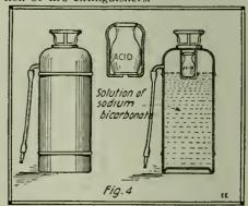
Section Thru a Standard Fire Extinguisher.
