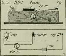
Simple Blinker Signal Set to Ald in Learning the Code, with Lamp and Buzzer.
