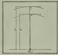
Fig. 7. Here Two Masses m-m, Are Considered as Condensed Into Points, Attached to Weightless Strings of Different Radil. If Both Strings Are Cut, and the Masses Considered as Joined, Then There Will Be No Rotation About the Common Center of Gravity.
