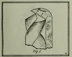
Using Grinding Gage to Test Edge of Twist Drill When Sharpening It.
