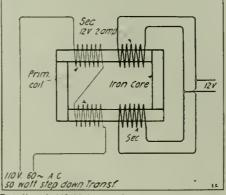
Details of 110-Volt to 12-Volt A. C. Transformer. Secondary Colls May Be Connected in Parallel or in Series.
