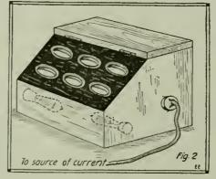
A 110-Volt Two-Lamp Egg Candling Cabinet with a Capacity of Six Eggs. It Can Be Easily Built by Anyone or Purchased as Desired.
