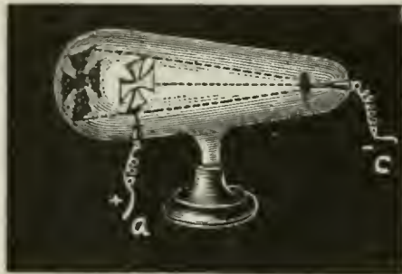
Fig. 95-A. Vacuum Tube for Demonstrating That Cathode Rays Cast a Shadow. The Rays Travel in Straight Lines, as the Metal Cross and Its Shadow Prove.
