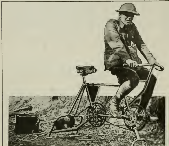
The Above Illustration Shows an Ingenious German Method of Generating Electricity for a Wireless Installation in the Trenches, Captured in a British Advance. A tandem bicycle with its wheels removed has been fixed to the ground, and the pedal wheels connected by belting with a small dynamo.
