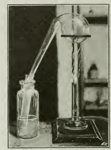
Fig. 138—Retort Method of Preparing Bromin from Potassium Bromid, Manganese Dioxid and Sulfuric Acid.
