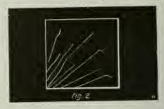
The Paths Taken by "Alpha Particles" in Air—After Photograph Taken by Wilson with the Arrangement Described and Illus-trated at Fig. 1. Alpha Particles May Travel 12 Centimeters Thru Air.
