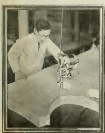
The Cutting Division of the Red Cross Does Its Work by Electrical Machinery. After the Pattern of the Garment is Stencilled Many Thicknesses of Cloth Are Cut at Once with Motor-Driven Cutters of the Type Here Shown.
