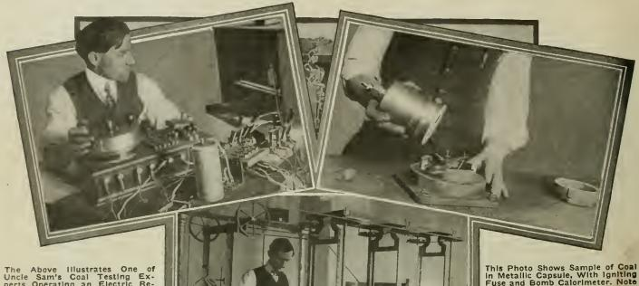
The Above Illustrates One of Uncle Sam's Coal Testing Experts Operating an Electric Resistance Bridge Connected With the Bomb Calorimeter.
