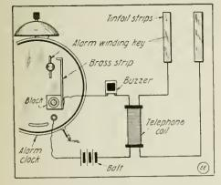
Are You a Commuter? An Ingenious Experi-menter Has Perfected a Sure-Fire Electric Ejector for All Such. Simply Connect the Circuit-Closer to Your Clock; Hook Up a Buzzer, and Telephone Induction Coil as Shown and Also Two Tinfoil Strips, Laid Under the Sheet. When 5 A. M. Arrives, You Will Awaken—Never Fear.
