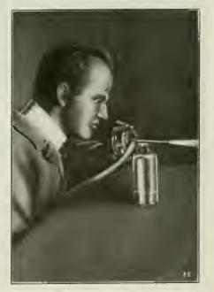
Fig. 90. Another Sodium and Water Experiment—After the Action Stops the Air Orifice of a Bunsen Burner Is Heid Over the Bottle, Giving a Yellow Color to the Flame.
