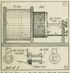
A Good Way to Build Dust-Proof Coupler Switches. The Square, Revoluble Shaft Turns the Sleeve to Which the Switch Blade Is Attached.
