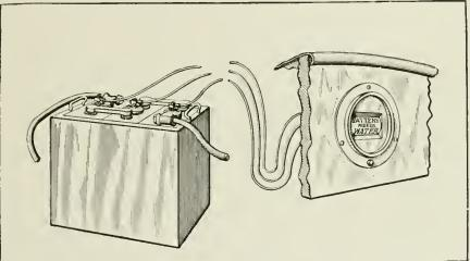
Every Battery User, and That Includes Most Every Autolst, Knows What a Nuisance It Is to Keep Tabs on the Electrolyte Level. Here's An Instrument That Indicates Instantly When "Battery Needs Water."
