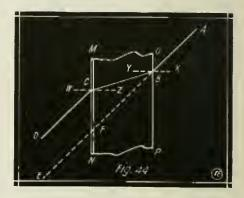
Diagram Illustrating How a Beam of Light Is Bent or Refracted, as A, B, C, D, In Pass-ing Thru a Piece of Glass M, N, O, P.
