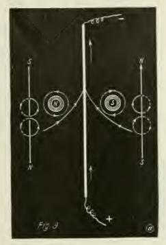
How the Author Explains the Action of a Magnetic Needle (Compass) When Placed in the Field of a Charged Conductor.
