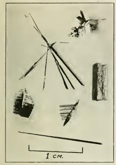
Fig. 1. A Few Specimens of Extra Sensitive Selenium Crystals Used by Professor Brown in His Researches on the Electrical Action Occurring in This Substance.
