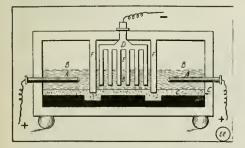
Fig. 88. Diagrammatic View of the Castner-Keliner Process for the Electrolytic Production of Caustic Soda and Caustic Potash.
