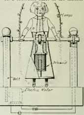
illustrated. A small motor mounted in the base of the toy connects with the revoluble shaft by means of a belt; the motor circuit being periodi-cally made and broken at the proper instants, by the contact disc and brushes carried on one end of the shaft. When the skip rope reaches the downward position, the toy fig-nre is pulled upwards by means of the solenoid concealed in the skirt.
