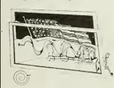
the front of cabinet shown, has for instance a waving flag painted on the face of it. Back of this screen there are placed several lamps for illumination and in front of this a slowly revolving metal spiral con-nected to a small electric motor. For best results the space around the flag should be made opaque. The spiral is cut out from a flat piece of metal and afterward expanded to the shape shown in the cabinet.
