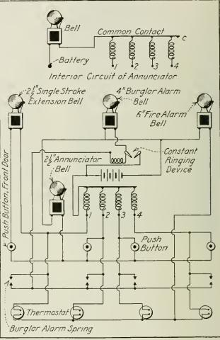
Hook-up for Combined Call Bell, Fire and Burglar Alarm System with Centralized Battery.
