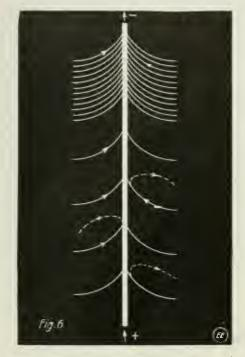
Interesting Chart of the Motions Followed By a Suspended Magnetic Body Near a Charged Conductor: the Body Moves In-ward Toward the Wire as Well as For-ward, Thus Proving the Existence of Currents Moving Inward and Forward. in the Direction of the Current.
