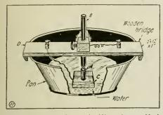
A Novel Experimental Microphone Made With a Pan of Water and Two Carbon Rod Contacts, One of Which Floats on the Water As Seen.
