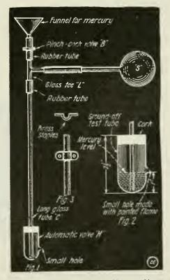
Important Features of Ideal Mercury Vacuum Pump for the Experimenter, Including Details of Automatic Over-flow Valve.
