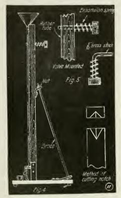
Side View of Home-made Mercury Vacuum Pump Which is Suitable for Exhausting Geissler Tubes, X-ray Bulbs, Lamps, Coherers, and a Host of Other Things Dear to Every Experimenter's Heart.
