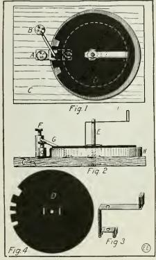
Home-made Code Transmitter Constructed from Cardboard Disc, a Hand Crank to Turn it with and a Contact Spring Which Closes the Sounder or Buzzer Circuit.
