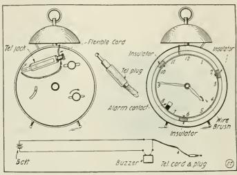
By Employing a Telephone Jack Switch as Shown, It is Possible to Disconnect the Electric Alarm Attachment from the Clock In-stantly. A Very Desirable Feature.
