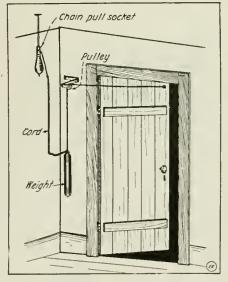
It Is Often Desired to Have a Door Control a Lamp, Such as in Cellars, Garrets, Etc. By Attaching a String and Counterweight to a Chain-Pull Socket, the Problem Is Solved.
