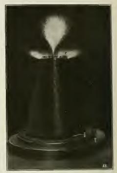
Fig. 1. Illustrating the Vigorous High Frequency Discharge From Free Electrode, As Well As Top, of Oudin Coll of Good Design.
