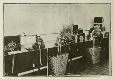
Fig. 2. This Picture Shows One Corner of the Operating Room of the Trans-Atlantic Cable Office at Penzance, England. The Perforated Paper Tape Passes Thru the Automatic Transmitters Which Send Out the Dots and Dashes Thru the Cables.
