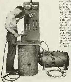
Complete Electric Arc Welding Outfit. It May Be Moved From Job to Job When Desired. Note the Glass Shield Which Operative Uses to Protect Eyes From Blinding Glare.
