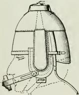
theing fitted with two telephone re-ceivers pressing against the ears, use is made of a single telephone re-ceiver mounted at the top of the helmet. This communicates with two sound channels which extend downward on either side of the helmet to the ears. The microphone is adjustably supported on a remov-able bracket, pivoted on either side of the helmet in the manner shown.
