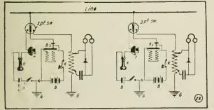
A Clever Scheme Permitting Telephone, Telegraph or Radio Messages to be Transmitted and Received Over a Telegraph or Lighting Circuit.
