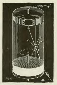
The Well-known Experiment of the Revolving Wire Dipping in Mercury, Is Used to Further Prove the Author's Case of "Currents About Magnets."
