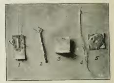
Some Specimens of the Work Accomplisht by New Aluminum Solder. The Joint is as Strong as the Stock.
