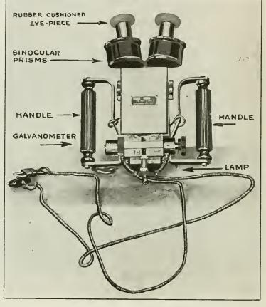
Here is the Latest Teutonic War Device. It Permits the Radio Operator in a Flying Machine to "See" the Wireless Signals. Thus the Engine and Other Nolses Do Not Bother Him In the Least.
