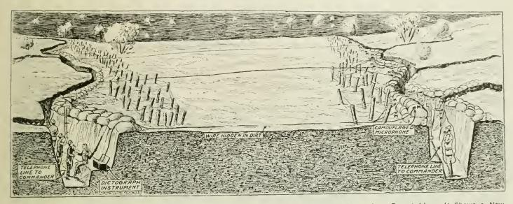
Listening to the Doings in the Enemy's Trenches By Means of Supersensitive Microphones Is a Recent Idea. It Shows a New Way How to Get Advance Information, as. for Instance, Just When the Enemy Intends to Attack, Etc., Etc.
