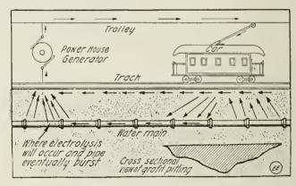
Diagram Showing How the Street Rallway Current Often Strays from the Ralls to a Water Pipe, Eventually Causing a Ruptured Main Where the Current Leaves the Pipe Line.
