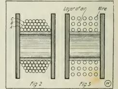
Fig. 2 Shows a "Staggered" Radio Inductance and Fig. 3 a Sectional View of the New "Morecroft" Multilayer Radio Winding, Designed to Have Minlmum Distributed Capacity.
