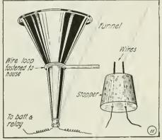
An Electric Rain Alarm Is of Undoubted Value in Every Home. The Rain Water, Mixing With a Few Grains of Salt, Closes the Alarm Circuit.
