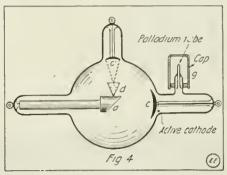
Special Form of X-Ray Tube of the Single-Focus Type, Fitted With Palladium Vacuum Regulator and Focussing Mirror "C", Also Copper Cone "d," for Dissipating Auxiliary Cathode Stream.
