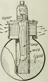
perforated tube surrounds the lamp, the tube itself being covered with an absorbing wick. In this way the liquid is spread out so as to realize the full vaporizing benefit from the heat of the lamp, and the vapor escapes thru the perforated ring at the top of the device as shown by the arrows.
