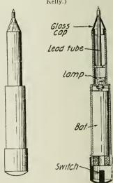
A useful invention comprising a suitable casing containing a miniature dry cell, small tungsten lamp, and means for holding the pencil lead as well as a switching device. To open or close the lamp circuit, the sliding cap at the end of the pencil is moved into or out of contact with the lower end of the dry battery.
