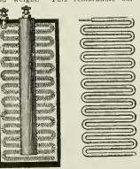
terial such as bibulous paper, and then bent or corrugated as shown in a sinuous form. The zinc is first perforated so that the carbon cathode can pass thru the various undulations of the encased zinc ele-ment without touching the zinc it-self.
