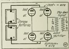
Proper Connections for Electrolytic Rectifier and Step-down Transformer.
