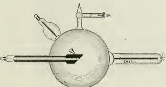
Commercial Form of a Second Type of Single-Focus High Frequency X-Ray Tube Shown Sectionally in Fig. 4. These Tubes Are Adapted to High Power Testa or Oudin Colls.
