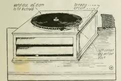
A Toothed Metal Disc Driven By a Phonograph Motor So As to Interrupt the Condenser Circuit Rapidly Provides a Serviceable "Tikker."
