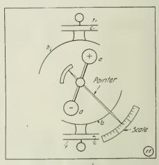
Connection and Principal Parts of Electrostatic Voltmeter Such As Used in Measuring High Potentials.
