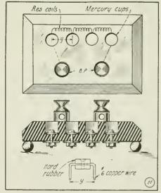
Simple and Efficient Variable Shunt for Use With Galvanometers, Employing Mercury Switch.
