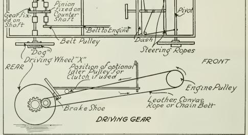
Why Wish for a Flivver-ette, "Bugs"? Here's How to Make One From the Simplest Materials Possible. Four Wheels, a Few Sticks of Wood, a Broom-stick, a Battery and Spark Coil, and Lastly—a Discarded Motorcycle Engine That Still Peeps, and You're In for the Tim^ of Your Life, Even to Stealing Your Rival's Best Girl.
