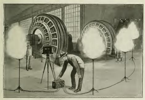
A New Photographic Scheme Involving the Application of Electricity to Rotate a Panorama Camera and to Ignite a Series of Flash-Lights Successively and At the Proper Instant. In This Way an Even Illumination of the Scene Is Assured.
