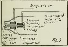
Details of "Holding" and "Telegraphing" Electro-Magnets of Electric U-boat "Blood-hound."
