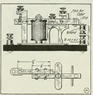
Substantial Design of Heavy Current Relay Key Which Can true for the air space coils,
