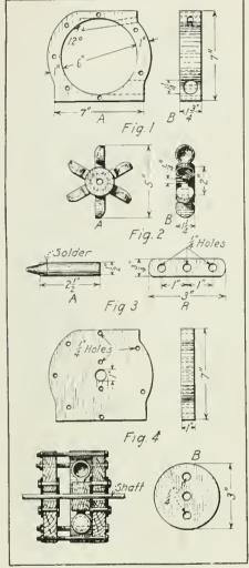
Construction Details for a Small Water Motor Which Will Prove Useful in Driving Dynamos or Other Light Machinery.
