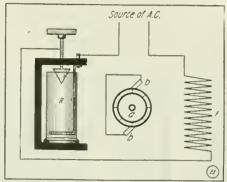
A Plan Whereby a Small D.C. Motor Can Be Operated As a "Repulsion" Type Motor On A.C. Circuits. Shift the Shorted Brushes Until Best Results Are Obtained.
