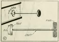
To Prevent "Body" Capacity Interfering With Undamped Wave Audion Tuning Use May be Made of This Extension Handle.
