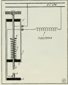
This Electric Gas Lighter Will Be Found a Distinct Convenience in Every Shop and Laboratory. Use an Iron Core Inductance On A.C. Circuits and a Resistance Coil On D.C. Circuits.
