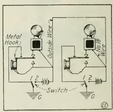
To Make This Simple Telephone System All You Require, Are Two 75 Ohm 'Phones, 2 Call Bells, 2 Push Buttons, Batterles, 2 Switches and a Pair of Home-made Hook Switches,
