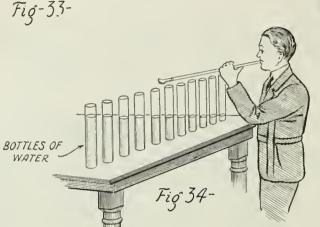
Fig. 33 Illustrates the Well-Known Tin-can Telephone, Which Shows the Principle of Sound Conduction by Means of a Vibrating String. Fig. 34 Shows the Principle of the Organ Pipe. The Air Columns Are Set in Vibration by Blowing Over Them.
