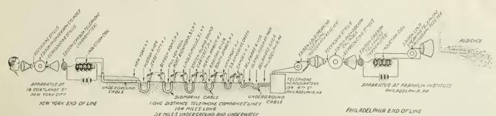
One of the Most Remarkable Telephonic Demonstrations Ever Attempted Is That Here Illustrated. By Means of Phonographs and Loudspeaking Telephones the Human Voice Was Transmitted Thru a Series of 48 Physical Changes, 15 Different Mediums and Thru the Air 5 Times, Between New York and Philadelphia. Mr. Hammer, Who Engineered This Stunt, Was Awarded the "Franklin Medal" in Honor of the Occasion.
