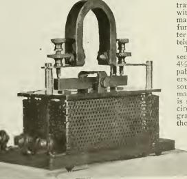
Something New in Telegraph Sounders—One That Actually Works Efficiently On Low Voltage Alternating Current From a Step-down Transformer.
