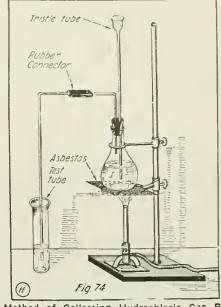
Method of Collecting Hydrochloric Gas By the Downward Displacement in a Dry Test Tube. See Experiment 79.
