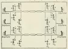
Schematic Diagram Showing How Three Telephone and Eight Telegraph Messages Are Transmitted Simultaneously Over Two Telephone Circuits. The A. T. and T. Co.'s Method.
