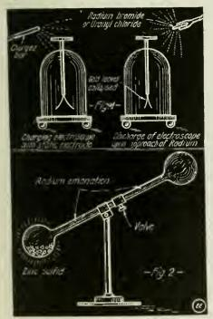
Top:—Discharging an Electroscope by Radium. Lower Illustration Shows a "Radium Light" Which Will Give Sufficient Illumination to Read By.
