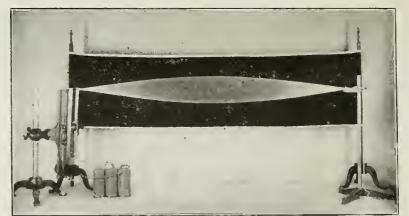
Interesting View of a String Vibrating in a Single Loop, Corresponding to a Simple Tone of a Fundamental Only. An Electrically Vibrated Tuning Fork Is Used in This Experiment.
