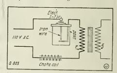
Simple Electrolytic Interrupter for Use on Alternating Current Circuits with Spark Coils or Open Core Transformers.
