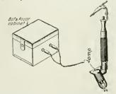
so that one may see at all times on any part of the face, which is is usually difficult with the ordinary source of illumination, due to shadows. She also provides a neat combined razor and battery cabinet, the lower part containing a suitable dry battery, with a flexible cord to connect the miniature lamp with the battery. A new battery may be quickly placed in the cabinet by means of a sliding bottom. The device would seem of extreme value to all military and traveling men.
