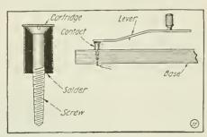
Save Your Cartridge Shells, Boys. They Make Good Switch Points, if a Wood or Machine Screw Is Firmly Embedded in the Shell by Means of Solder. The Leads May Be Soldered to the End of the Screw.
