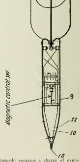
torpedo contains a charge of explosives to be detonated by an electric fuse 10-11, operated by switch 15, when the missile strikes its target. The inventor provides an "attraction" electro-magnet 9, suspended to swing in any direction.
