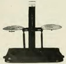
Every Experimenter Needs a Small Balance for Weighing Chemicals On. Here's One Made from a Telephone Ringer Frame Fitted with a Set of Pans and a Scale.
