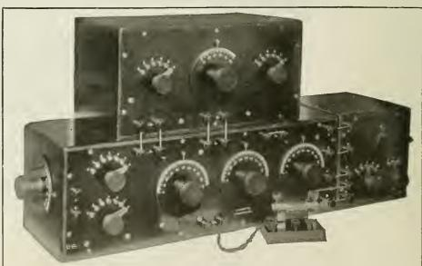
Fig. 2—An Excellent Audion Type Radio Receptor for "Mosquito Fleet" Service.
