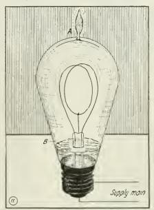
A Novel Experiment with an Incandescent Lamp Which Is Filled Up to "B" with Gaso-line. When Connected to Live Circuit Gas Is Generated and May Be Ignited at A by a Match.
