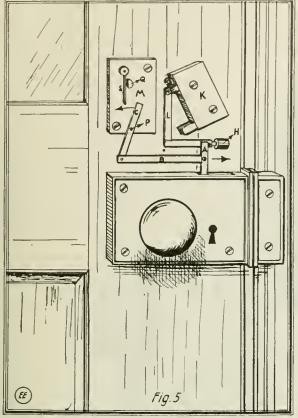
Arrangement of Interlocking Switches for Con-"Stick Relay" in Burglar Alarm System Here Described.
