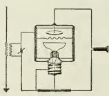
metal sleeves placed inside and outside of the tubular glass bulb. The inner sleeve supports the usual grid and is charged thru the glass dielectric from the outer sliding metal sleeve, connected in the circuit as shown.
