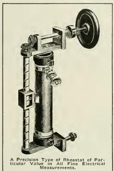
resistance such as the one illustrated. This particular rheostat is of English manufacture and comprises a metal tube covered with insulation and over which many turns of closely wound bare resistance wire are
