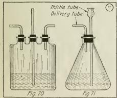
At Left—A Wolff Bottle With Three Necks: At Right—Erlenmeyer Flask Which May Bo Substituted for the Florence Flask Specified.
