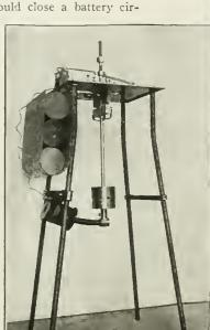
plunger was moving into the solenoid the flux threading the latter was increasing at a rapid rate, due to the decreasing refuetance of the magnetic circuit, the magneto-motive force meanwhile remaining con-stant. This change of flux induced a volt-age in the turns of the solenoid which tended to oppose the E.M.F., which was forcing the current thru the coil; in other
