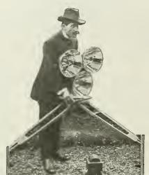
luminous rays are concentrated in a very small point or space. The tungsten lamps employed are of Dussaud's own design. Some of them are only 0.8 to 1.6 inches in radius. Groups of three are used in some models. They are successively flashed in the focus of a condensing lens, without breaking down the filament or blackening the bulb. Indeed, it is said that the results produced are identical with those obtained with an electric arc ten times more obtained with an electric arc ten times more
