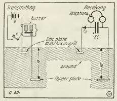
An Effective "Buzzer" Telegraph System Which Employs Two "Ground" Plates at Each Station, Each Plate Buried at a Different Level. A Radio Detector, Fixt Condenser and Telephone Receiver Are Used at the Receiving Station.
