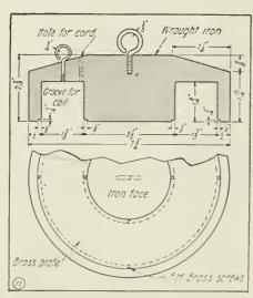
Something Everyone Finds a Need for at Some Time Is a Good Lifting Magnet. Here Are the Details for Building an Efficient 12-Ton Electro-Magnet for Use on D.C. Circuits.
