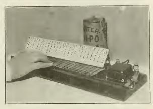
The "Simplograph"—An Attempt to Make the Learning of the Telegraph Code as Simple as Possible. A Buzzer Sounds the Signals for Radio Students.
