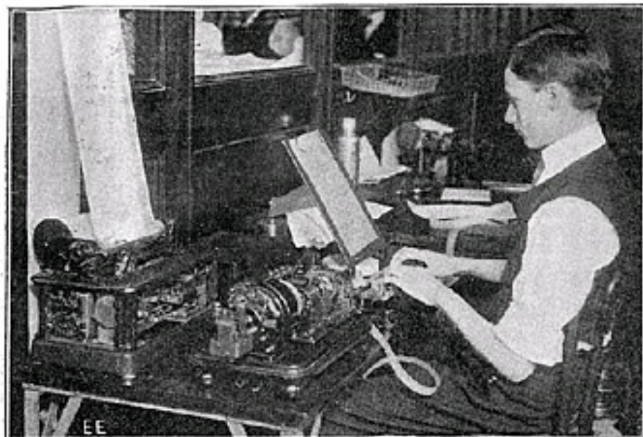
Photo (C) by Underwood & Underwood. Showing Morkrum Sending and Receiving Printing Telegraph System Installed in Associated Press Office in New York City. Local Printer to Left.
