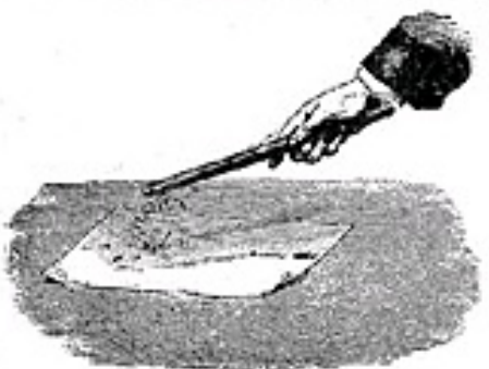
Illustrating the First Principle of Electricity. The Electrified Stick of Sealing Wax.
