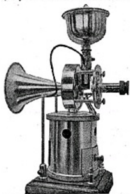
Fig. 5. The Carbon Grain Stream Microphone.
