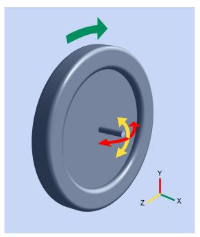
**Figure 9-1** In a traditional gyroscope, a wheel that is rotating (shown by the green arrow) will resist a turning force on either of the axes (shown by red and yellow arrows) perpendicular to its axis of rotation.
