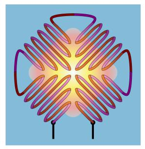
**Figure 28-2** Simplified diagram of the thermopile configuration inside an infrared sensor chip. Radiation arriving through a window in the chip affects the thermocouple junctions in the central region, while junctions around the edges remain at a lower temperature.
