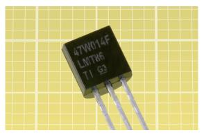
**Figure 27-13** A sample of the LMT86 CMOS temperature sensor. The background grid is in millimeters.
