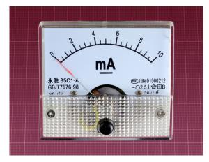
Figure 30-1 A traditional-style analog ammeter.
