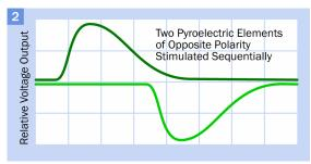
**Figure 4-4** Top: in a pyroelectric detector, if a change in temperature affects two elements of opposite polarity simultaneously, their voltages cancel each other out. Bottom: if one element is triggered before the other, the detector emits a signal.
