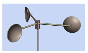
**Figure 19-1** The basic design of a metereological cup anemometer.
