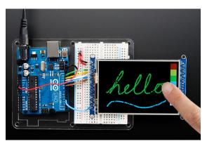
Figure 14-2 An Arduino-compatible touch screen mounted on a breakout board, available from Adafruit.
