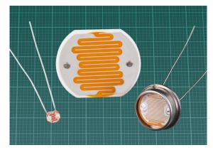
**Figure 20-3** Photoresistors are available in a wide range of sizes. The component in the center is shown at the same scale as the others. Generally speaking, larger components are able to conduct higher currents. The background grid is in millimeters.
