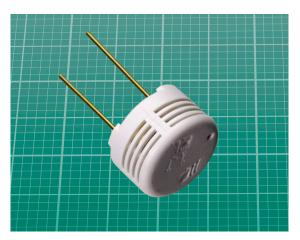
**Figure 18-4** A Humirel HS1101 humidity sensor. The background grid is in millimeters.
