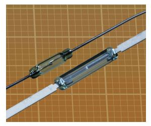
**Figure 3-11** Two SPST reed switches. Although the contacts may seem to be touching, in fact they are separated by a tiny gap, and these switches are the normally open type. The background grid is in millimeters.
