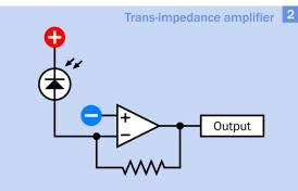
**Figure 21-7** Simplified op-amp circuits for use with photodiodes.
