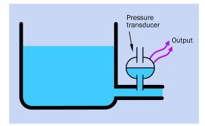
**Figure 15-10** A pressure sensor can assess the volume of liquid in a reservoir.
