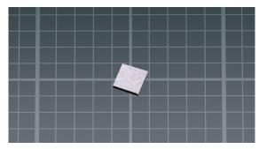
**Figure 28-3** A surface-mount infrared temperature sensor with digital output. Eight tiny solder pads are located on the underside. The background grid is in millimeters.
