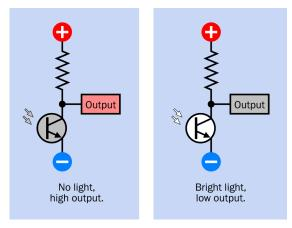
Figure 22-5 How an open-collector output works.
