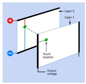
**Figure 14-1** Sections of a resistive touch screen are shown displaced for clarity. In reality they would be separated by a very small gap, allowing one section to make contact with the other in response to finger pressure.
