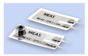
**Figure 11-4** Two versions of the LDTO-028K vibration sensor from Measurement Specialties, one with an added weight to lower its resonant frequency.
