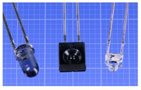
**Figure 22-1** A variety of phototransistors. The background grid is in millimeters. See text for details.
