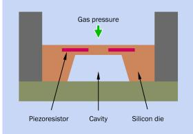
**Figure 17-2** A section of a flat-diaphragm pressure sensor, viewed from the side. An aperture in the top face of the chip allows air to enter. The sensor is etched into silicon, and the deflection of the wafer is measured using embedded piezoresistors.
