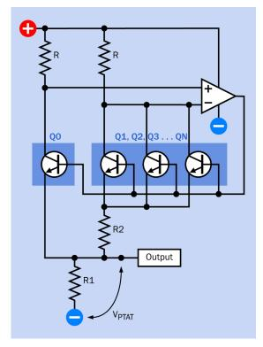
Figure 27-4 The Brokaw Cell. See text for details.
