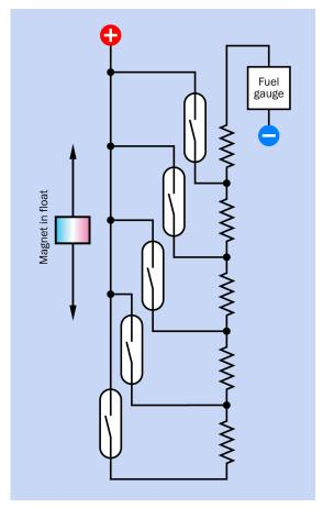
Figure 15-6 A float sensor with incremental output.
