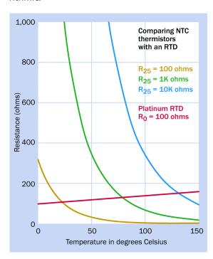
**Figure 26-1** The brown, green, and blue curves show the resistance of three generic NTC thermistors varying with temperature. The red line shows the resistance of a platinum RTD. Derived from a diagram created by Texas Instruments.
