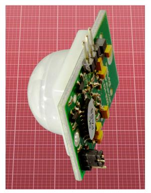
**Figure 4-10** A passive infrared detector mounted with basic necessary components on a small board.
