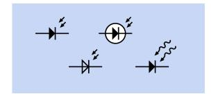
Figure 21-1 Symbols representing a photodiode.
