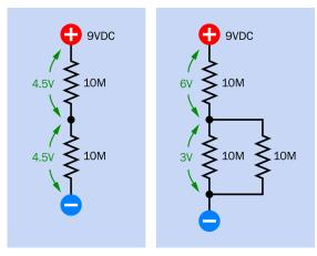
**Figure 31-5** If a meter measuring the voltage drop across a load has an internal resistance comparable to that of a load, the meter will not give an accurate reading. See text for details.
