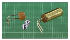
**Figure 8-4** At right, a tilt switch. At left, the cap removed, and the two balls that make internal contact. The background grid is in millimeters.
