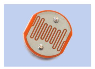
Figure 20-2 Closeup of a photoresistor. Two interlocking electrodes are mounted on a brown semiconductor laver.
