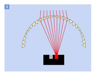
**Figure 4-7** Sections 1, 2, and 3 show fresnel lenses focusing an external source of infrared radiation on individual elements of a pyroelectric sensor.
