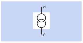
**Figure 27-1** A temperature sensor whose output consists of current varying with temperature may be shown in a schematic as a current source, using this symbol.
