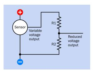
**Figure A-2** Using a voltage divider to reduce the range from a sensor.
