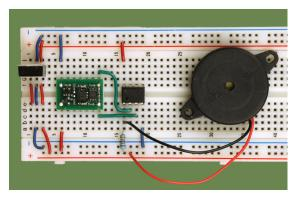
**Figure 10-4** Connecting the analog output from the DE-ACCM6G 2-axis comparator breakout board through a comparator to a piezo beeper.
