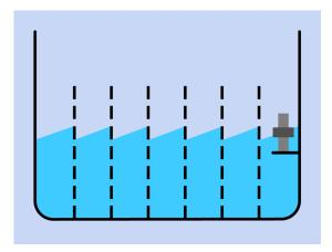
**Figure 15-11** Insertion of perforated baffles in a reservoir minimizes the sloshing that otherwise tends to occur when the reservoir is subject to lateral motion.
