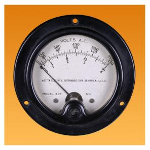
Figure 31-1 An antique analog volt meter.
