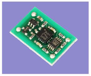
**Figure 10-3** A relatively early, relatively expensive breakout board using the 2-axis accelerometer LIS244ALH chip by STMicroelectronics. It has been superceded by chips that combine accelerometers, gyroscopes, and processors to provide a digital output.
