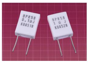
**Figure 30-6** Two current resistors manufactured by KOA Speer. Left: 0.1 ohms, 5W, 5%. Right: 1 ohm, 5W, 5%. The background grid is in millimeters.
