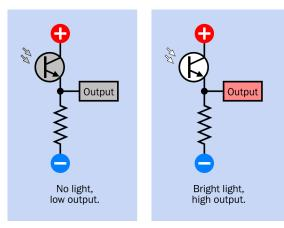
**Figure 22-6** Moving the resistor and taking an output from the emitter pin inverts the behavior of a phototransistor. Any device attached to the output must have a relatively high impedance to protect the phototransistor from excessive current.
