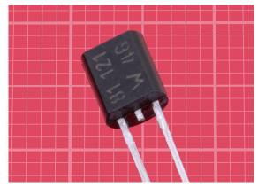
**Figure 24-1** A KTY81 thermistor from NXP. The background grid is in millimeters. Note the amputated center lead.
