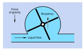
**Figure 16-2** In this configuration, friction on the rotor bearings is mitigated by taking advantage of the buoyancy of a low-density rotor in the liquid that passes through.
