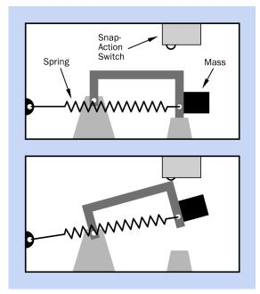
**Figure 11-5** A spring-loaded vibration sensor.
