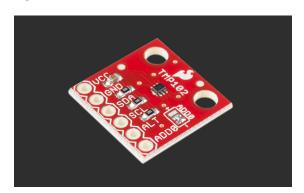
**Figure 27-11** The Texas Instruments TMP102 on a breakout board from Sparkfun.
