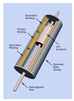
**Figure 6-7** Cutaway drawing showing the internal design of a linear variable differential transformer, in which the position of a sliding iron armature determines the voltage induced in the secondary windings.
