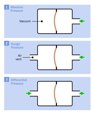
Figure 17-3 Three ways in which pressure is measured.
