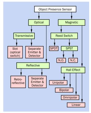
**Figure 3-2** Categories of object presence sensors discussed in this entry. Other types of object presence sensors exist, but are less common, and are not included here.
