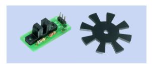
**Figure 7-8** A bare-bones optical encoder for DIY robotics.
