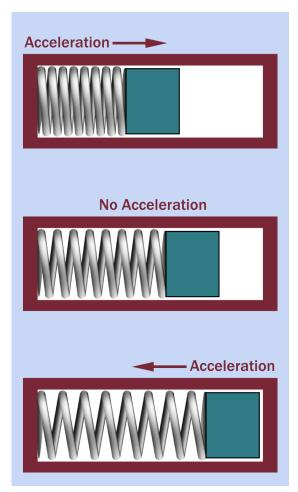
**Figure 10-1** Simplified view of an accelerometer consisting of a sealed tube (dark red outline) with a spring anchored to it at left. A small mass (dark blue) is attached to the right end of the spring. The mass responds to acceleration of the tube.
