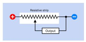
**Figure 6-1** A linear potentiometer can consist of a fixed track with a known voltage applied at each end, and a movable wiper.
