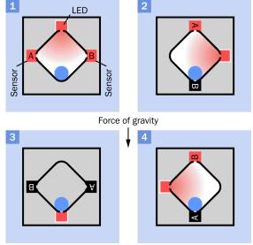
**Figure 8-10** The rolling-ball sensor inside the Parallax 28036. See text for details.
