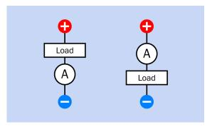
**Figure 30-4** Two options for placement of an ammeter in a circuit.
