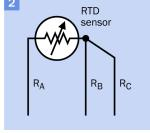
**Figure 26-4** A three-wire configuration enables temperature compensation for the leads to an RTD. See text for details.
