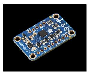
**Figure 10-6** This breakout board from Adafruit is built around an LSM9DSO chip that combines accelerometers with gyroscopes and magnetometers.
