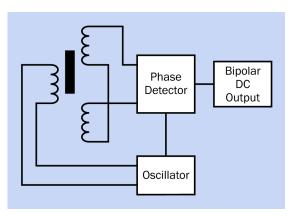
**Figure 6-8** Typical schematic for using a linear variable differential transformer.
