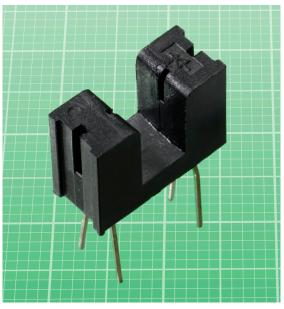
**Figure 3-5** A low-cost transmissive sensor, more commonly known as an optical switch. The background grid is in millimeters. The slot in the sensor is about 5mm wide.
