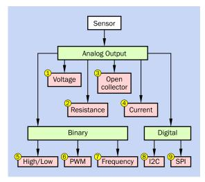
**Figure A-1** Nine possible types of output from sensors. The primary categories are highlighted in green.
