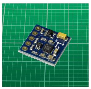
**Figure 2-1** The Honeywell HMC5883L 3-axis magnetometer mounted on a breakout board. The background grid is in millimeters.
