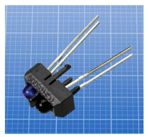
**Figure 3-9** The Vishay TCRT5000 retroreflective sensor. The background grid is in millimeters.
