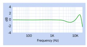
Figure 29-11 Frequency response for an electret microphone.
