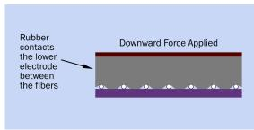
**Figure 12-10** In the top image, a flexible conductive layer is separated from an underlying rigid electrode by nylon mesh. In the lower image, a load applied to the flexible layer has forced more of it into contact with the electrode, reducing the resistance between them.
