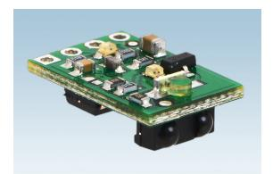
**Figure 3-6** The Vishay TSSP77038 installed with an appropriate light source on a breakout board from Polulo Robotics and Electronics.
