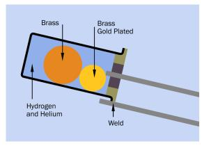
**Figure 8-2** Interior of the CW1300 tilt switch, from a scale drawing supplied by the manufacturer. The lower lead is welded to the shell of the sensor. The leads may be inserted in a circuit board.
