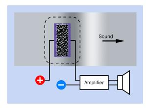
Figure 29-3 The principle of a carbon microphone.
