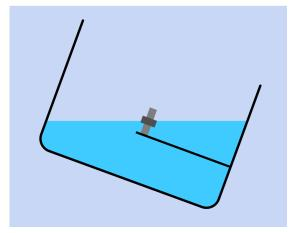
**Figure 15-12** If a float sensor is mounted centrally in a reservoir, it will be significantly less affected if the reservoir tilts.
