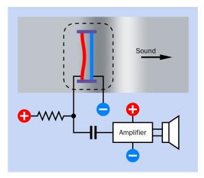
Figure 29-5 The principle of a condenser microphone.
