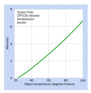
**Figure 28-5** Analog output from an infrared temperature sensor.
