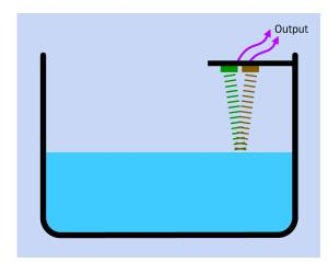
**Figure 15-8** An ultrasonic proximity sensor can measure the level of liquid in a reservoir.
