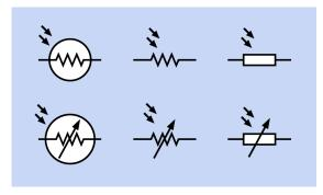
Figure 20-1 All six symbols for a photoresistor are functionally identical.
