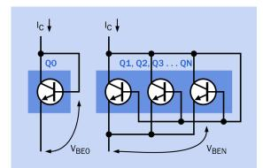
Figure 27-3 Comparing the base-emitter voltage of one transistor with a set of identical transistors can enable measurement of temperature regardless of the collector current and saturation currents, so long as all the transistors are at the same temperature. See text for details.
