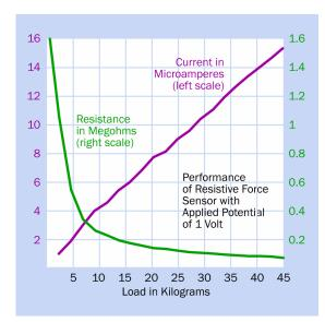
**Figure 12-11** The relationship between force, current, and resistance in a flexible resistive sensor, assuming a constant voltage of 1V is applied across it (derived from FlexiForce Sensors User Manual).
