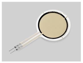
**Figure 12-8** A FlexiForce A401 resistive film sensor made by Tekscan, Inc. Its sensing area is 25.4mm in diameter (1 inch) and is rated to measure up to 111N (25lbs).
