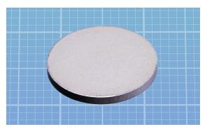
**Figure 24-9** This TDK B59060A0060A010 heating element is a PTC thermistor whose resistance rises rapidly around 80 degrees Celsius. Rated for 12VDC, it is intended for automotive applications. The background grid is in millimeters.
