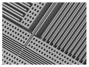
Figure 9-5 Electron micrograph of the STMicroelectronics LIS331DLH vibrating gyroscope installed in the Apple iPhone 4. The parallel plates at bottom-left function as a spring, while the elements at top-left and at right measure capacitance as their orientation varies according to rotational velocity. Photo courtesy of MEMS Journal published by Chipworks
