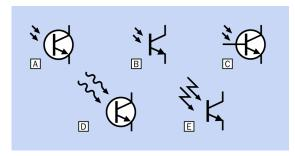
Figure 22-2 Schematic symbols for a phototransistor.
