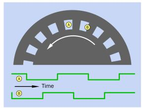
**Figure 7-6** With transmitter-detector pairs mounted at positions A and B, the phase difference between their pulse trains can show the direction of rotation of the wheel.
