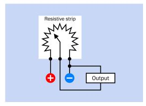
**Figure 7-1** An arc-segment potentiometer consists of a fixed track in the shape of an arc with a known voltage applied at each end, and a movable wiper.
