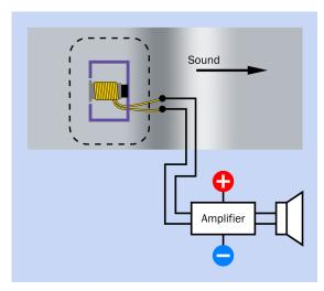
Figure 29-4 The principle of a moving-coil microphone.
