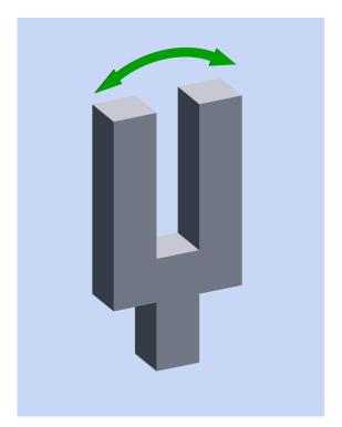
**Figure 9-2** A vibrating fork (green arrows) can be substituted for a rotating wheel in a gyroscope.
