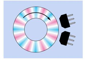
**Figure 7-14** Direction of rotation of the wheel can be deduced from the phase difference between the pulse trains from two sensors.
