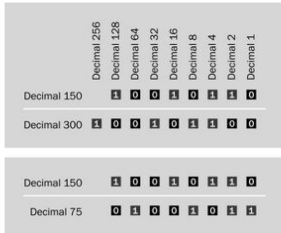
Figure 12-9. In the upper section of this diagram, a binary number represented by eight bits in a shift register is multiplied by 2 by shifting all the bits one space to the left. In the lower section, the same binary number is divided by 2 by shifting all the bits one space to the right. The binary values are shown in decimal notation to the left.
