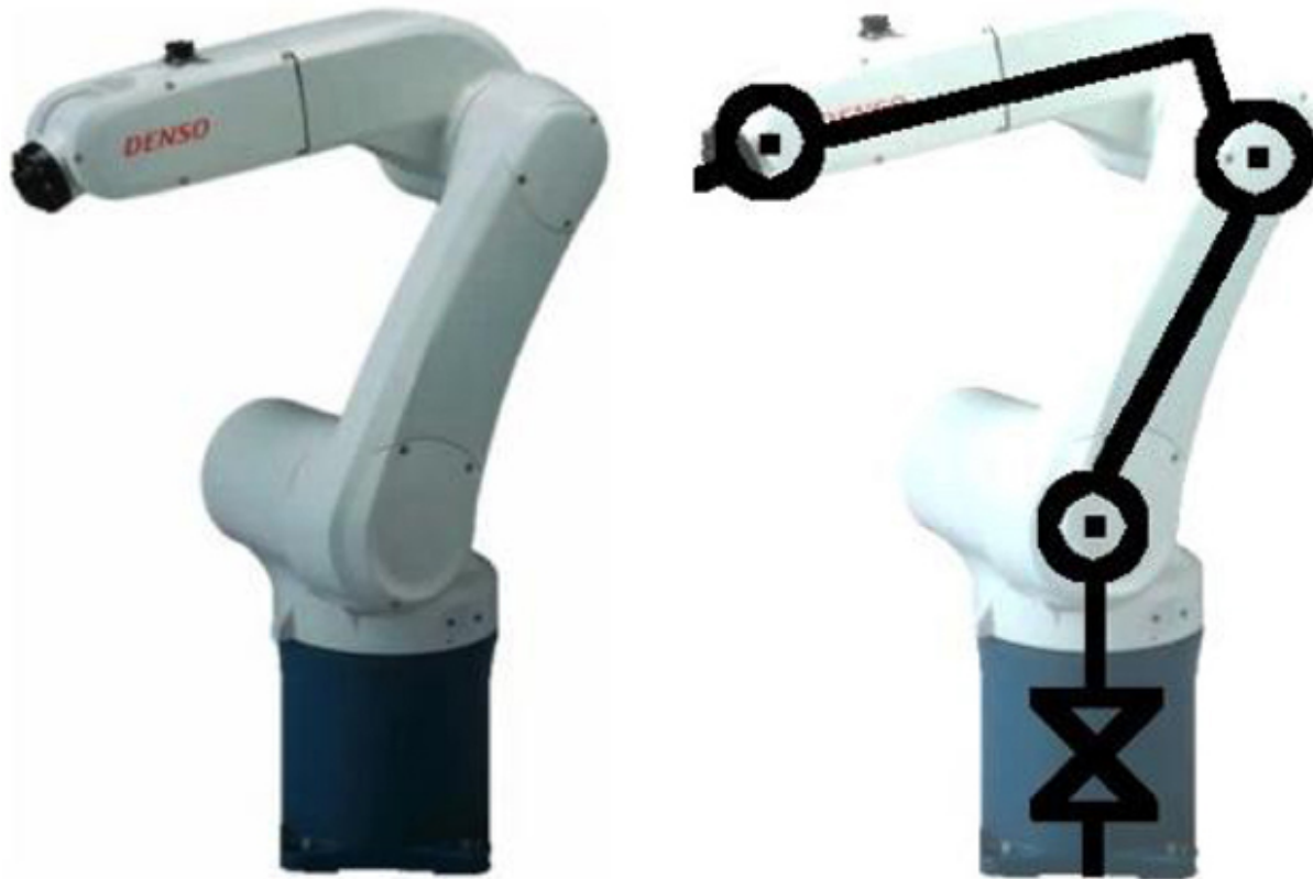
Figure 9-3 Free-body robotic arm with DH joint designations.
