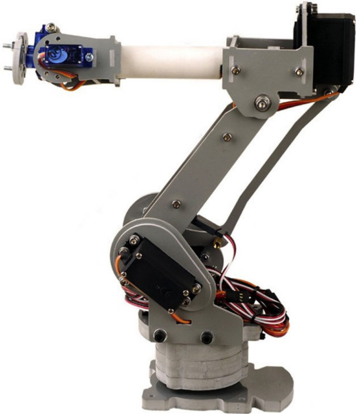
Figure 9-12 6-DOF SainSmart robotic arm.
