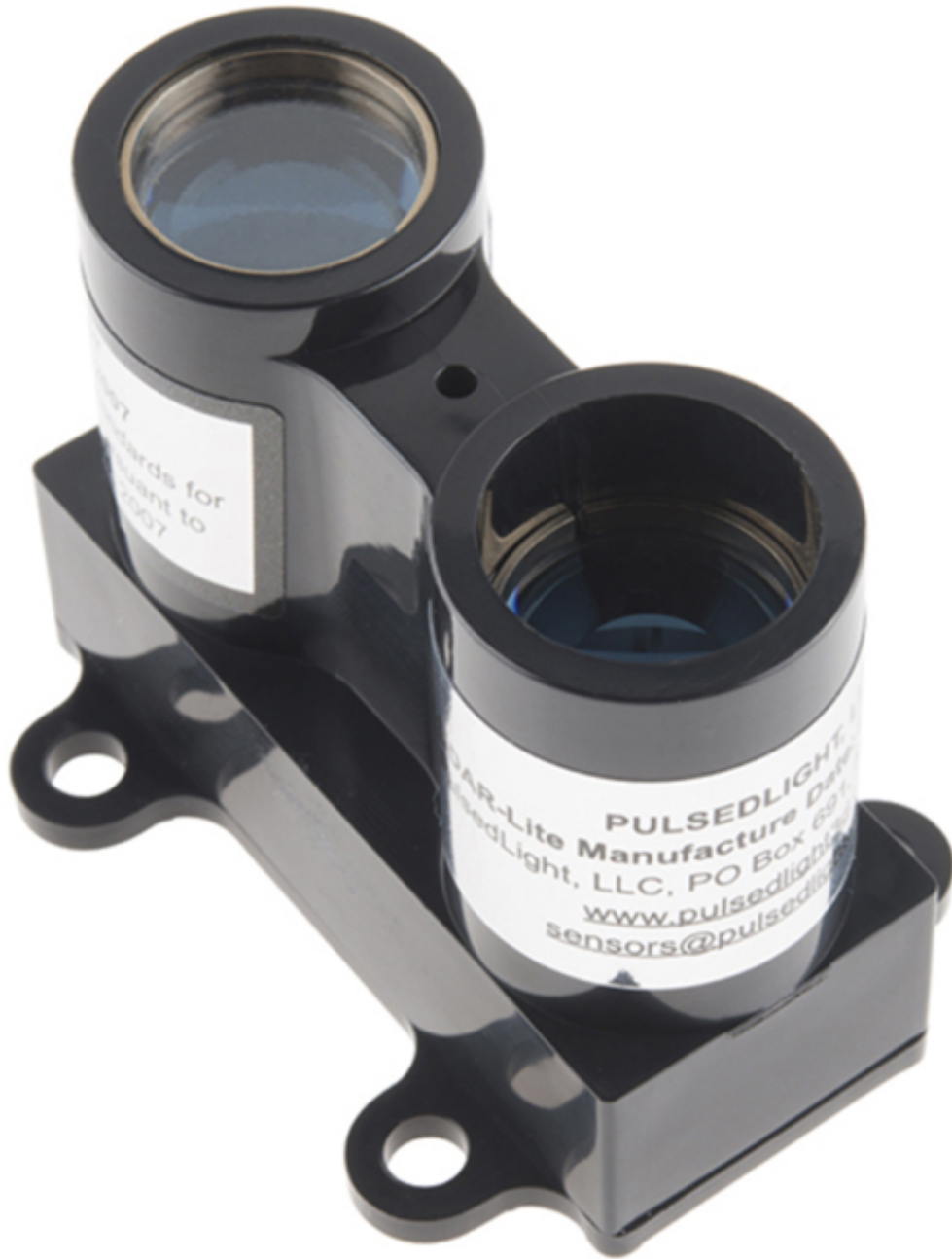
Figure 3-18 PulsedLight LIDAR-Lite sensor system.
