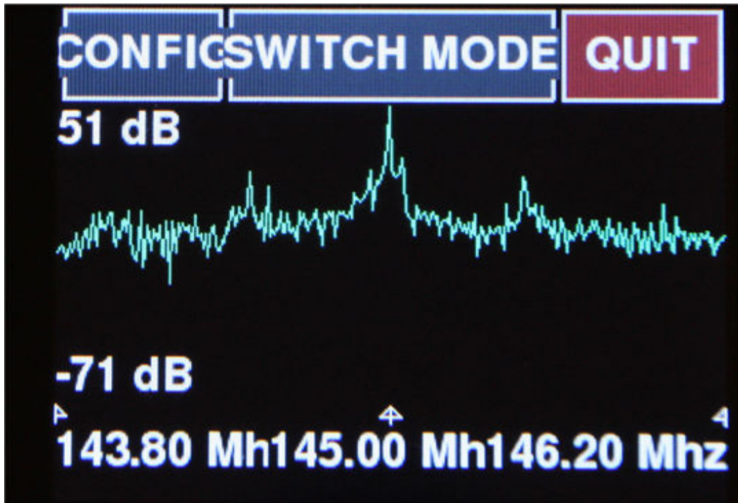
Figure 7-34 145.000-MHz CW transmission from an amateur radio transceiver.
