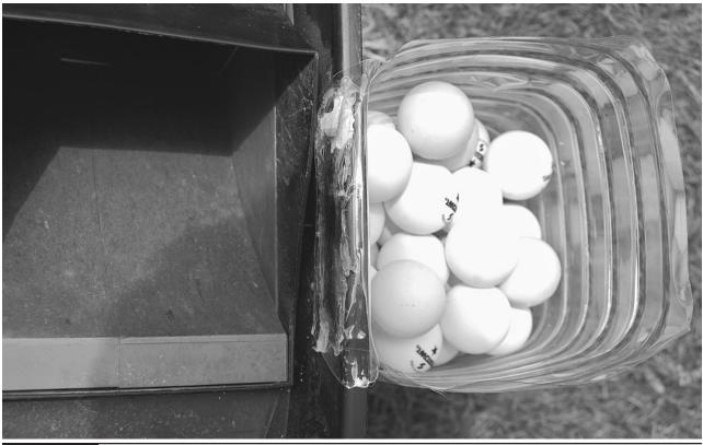
Figure 3-10 The magazine attached to the leaf blower
