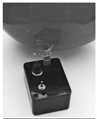
Figure 5-15 A balloon attached to the popper
