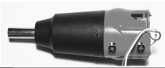
Figure 15-10 Sawn-off screwdriver
