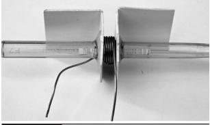
Figure 1-7 Winding the coil
