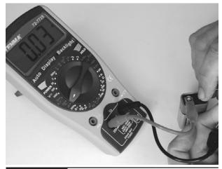
Figure A-8 Measuring current
