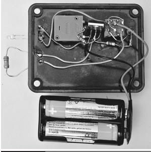
**Figure 5-13** The inside of the balloon popper, with all the components in place
