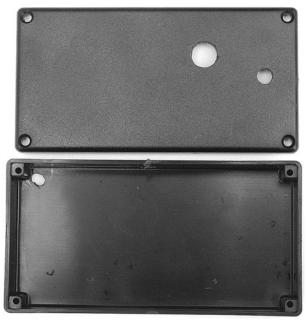
Figure 10-23 Drilling the transmitter box
