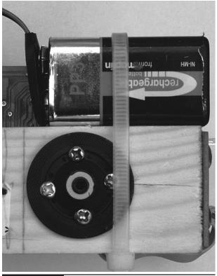
Figure 8-33Attaching the arm to the motor
