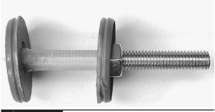
Figure 13-3 The bolt and homemade washers
