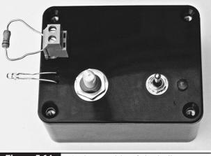
Figure 5-14Final assembly of the balloon<br/>popper
