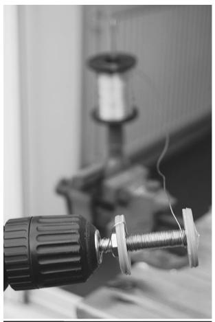
Figure 13-4 Winding using an electric drill
