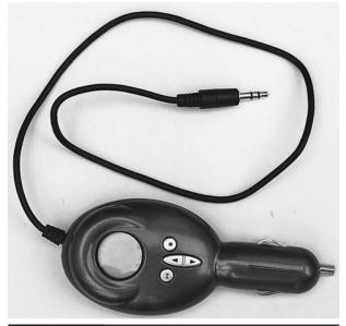
Figure 9-9 FM MP3 car transmitter
