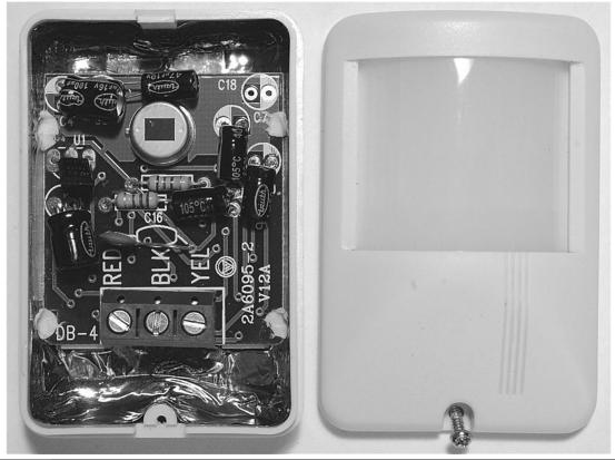
Figure 15-15 The PIR sensor
