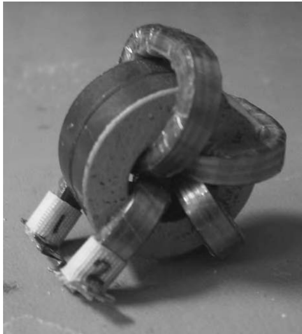
FIGURE 20.19 HF wideband transformer. (Courtesy MKS Instruments. Used with permission.)
