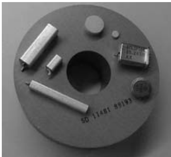
FIGURE 21.6 A picture of various resonators. From the left are three transmission line resonators for 500 MHz to 2 GHz operation, two dielectric resonators for 7 and 20 GHz operation, a 10 MHz crystal resonator, and a 300 MHz SAW resonator. The resonators are sitting on top of a 2.5 inch diameter dielectric cylindrical resonator for 850 MHz.
