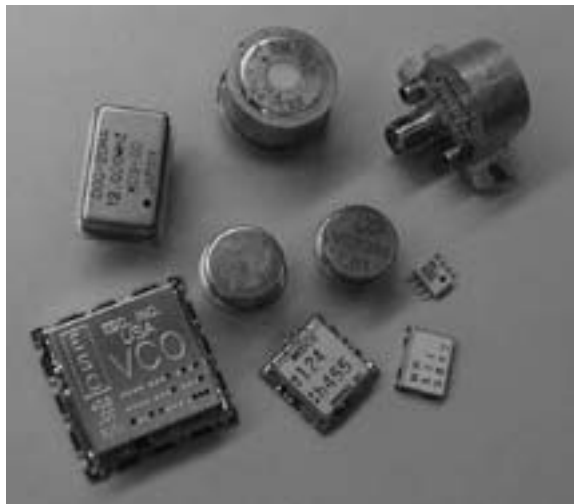
FIGURE 21.1 A picture of various RF and microwave oscillators. Top to bottom and across from the left there is a crystal oscillator and two YIG oscillators, two chip and wire oscillators in TO-8 cans, a microwave IC oscillator, and three discrete PCB VCOs in packages of decreasing size.
