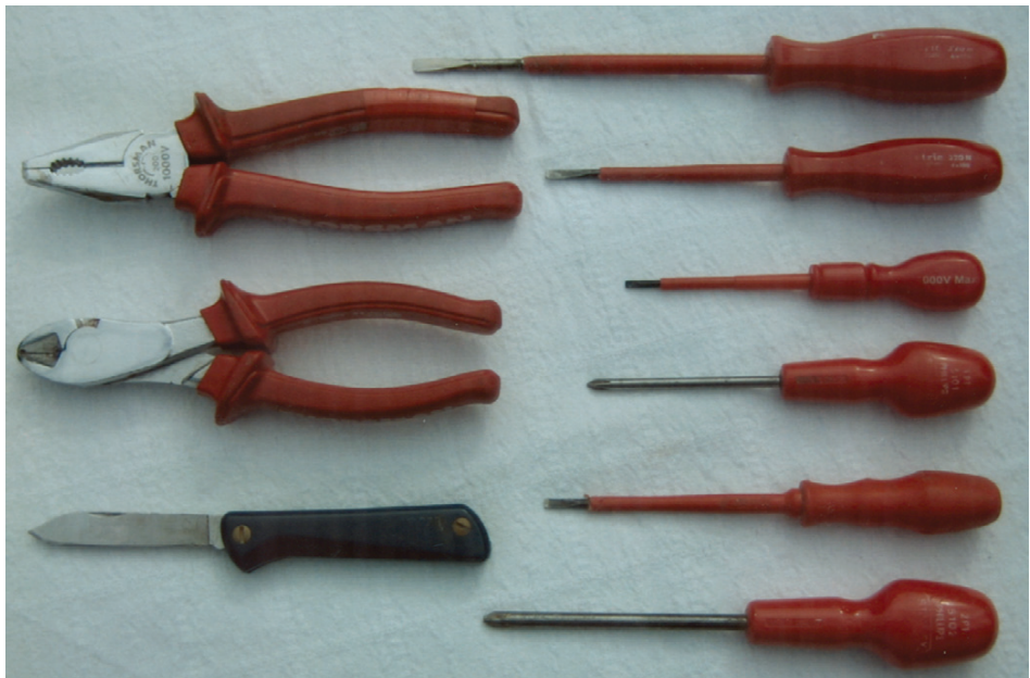
Figure 2.17 The tools used for making electrical connections.
