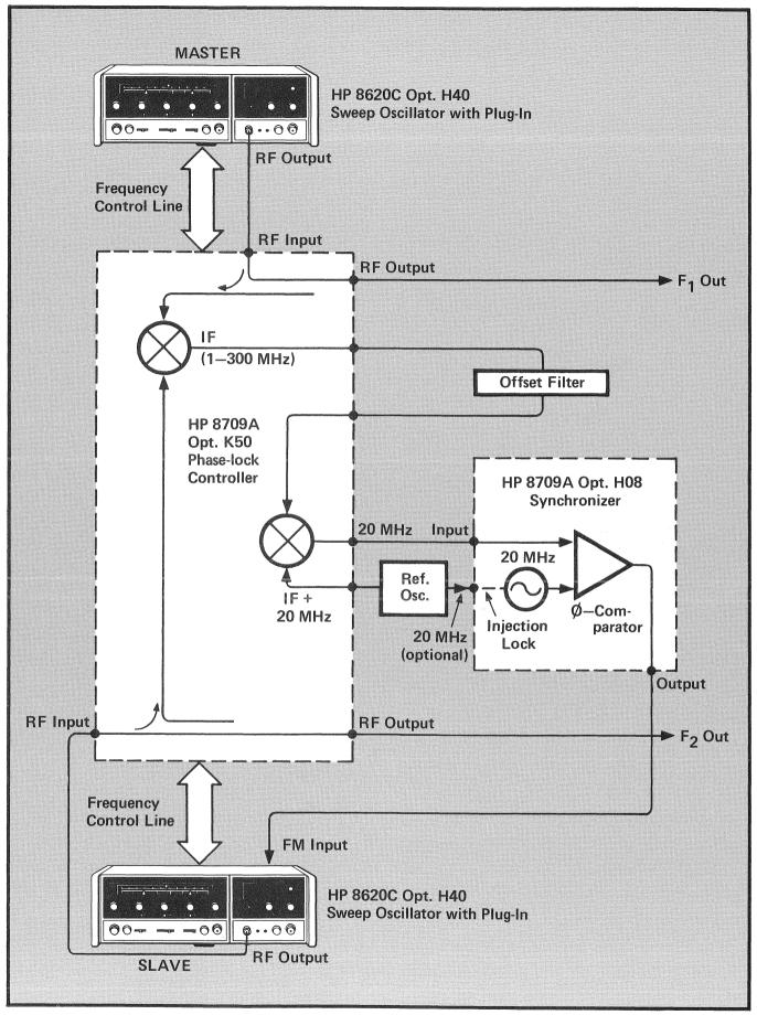
Figure 3. Two-Tone Sweeping Generator Block Diagram.
