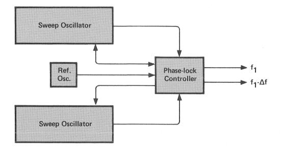
Designing and testing microwave mixers and receiver front-ends requires a local oscillator signal and the received signal, separated in frequency by the required IF. Broadband testing of such devices may be accomplished by taking CW measurements at discrete frequencies after manually tuning each of two signal sources. This method is both tedious and time-consuming, and it may result in the oversight of narrowband responses which occur between the discrete frequency points.
