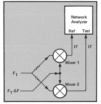
Figure 1. Mixer Test Set-up.
