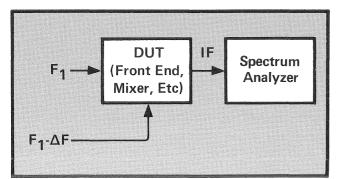
Figure 2. IF Signal Analysis Test Set-up.
