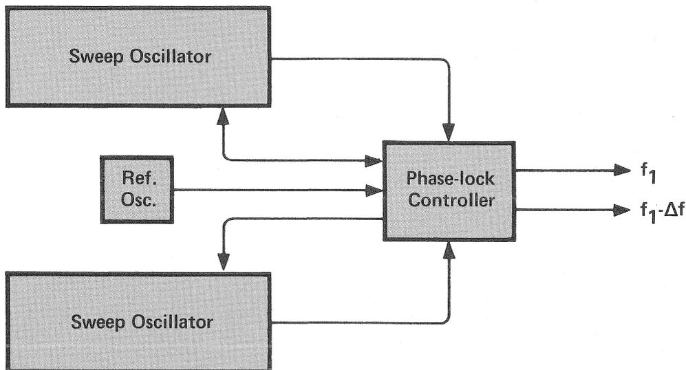
Designing and testing microwave mixers and receiver front-ends requires a local oscillator signal and the received signal, separated in frequency by the required IF. Broadband testing of such devices may be accomplished by taking CW measurements at discrete frequencies after manually tuning each of two signal sources. This method is both tedious and time-consuming, and it may result in the oversight of narrowband responses which occur between the discrete frequency points.
