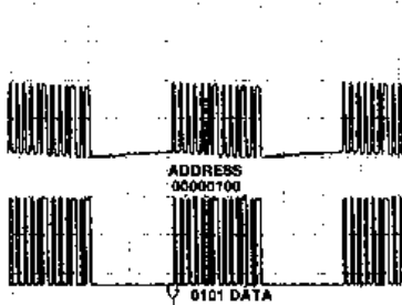
Figure 7.19 (a) SILRX-418-A receiver audio output (upper trace) and data output (lower trace) when receiving repeated 12 bit sequences of 0000 0100 0101. (b) SILRX-418-A pager application circuit treating all twelve bits as addresses, giving 4096 different possibilities
