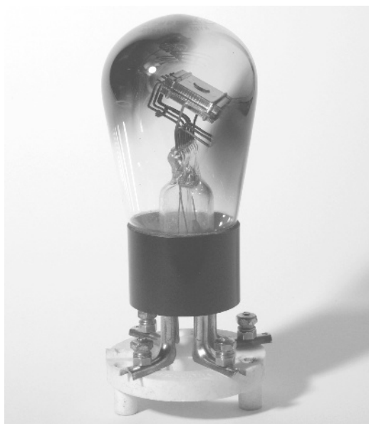
Fig. 4.25 P215 directly heated oxide-coated cathode valve
