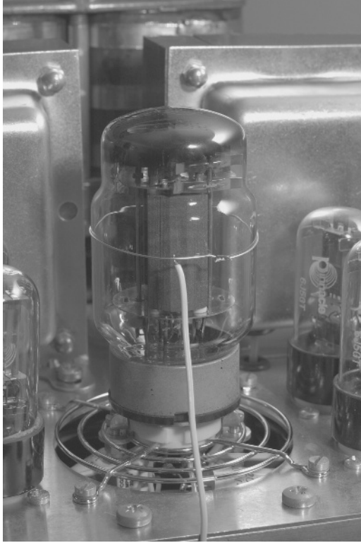
Fig. 4.37 Thermocouple bead clamped to valve by thin copper wire
