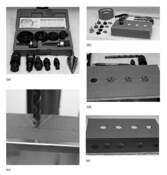
FIGURE 6.1 Chassis construction techniques: (*a*) selection of chassis punches for use with tube-based projects; (*b*) the chassis is covered with masking tape to facilitate marking of hole positions and sizes for the components; (*c*) use a drill press for precision cuts and control over the
