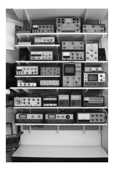
FIGURE 6.7 Test equipment for audio project construction and troubleshooting. (Observant readers will note that all of the test equipment in this shop is classic 1970s era Heathkit instruments, which seems appropriate for building classic tube amplifiers.)
