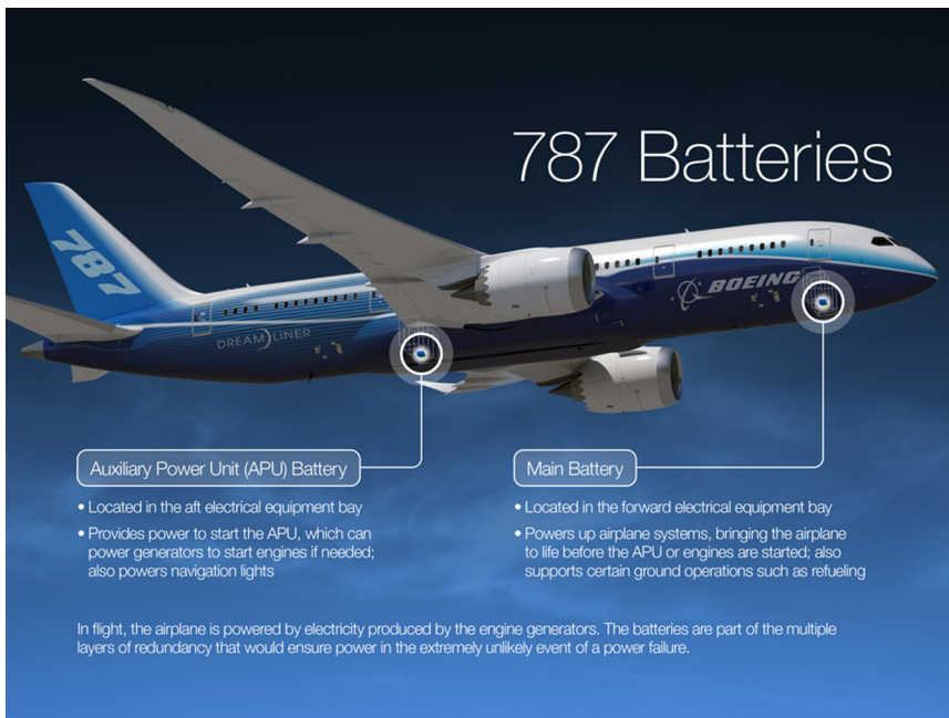
Figure 27 Boeing 787 lithium-ion batteries.
