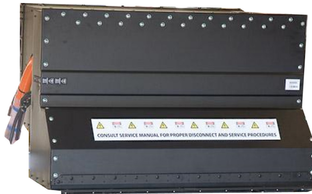
Figure 12 Tesla Roadster lithium-ion battery pack.
