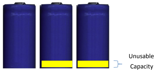
Figure 6 Imbalanced cells at end of discharge.
