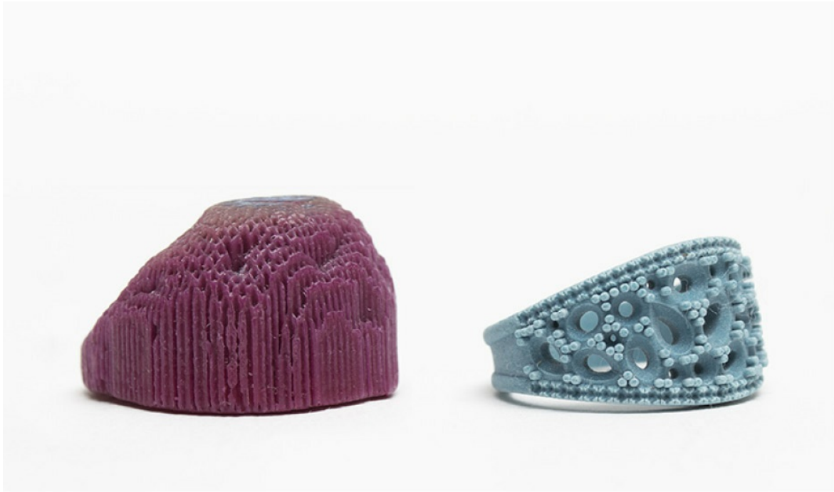
Figure 5.3 – DOD printers print dissolvable support (the part on the left) around wax parts used for investment casting allowing for the production of highly intricate details. The part on the right shows a wax ring once support has been removed
