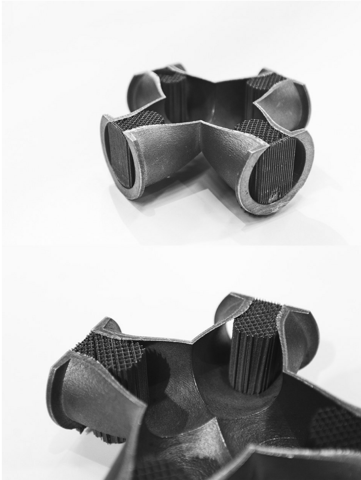
Figure 7.4 – An SLM print with support still attached showing the support lattice geometry
