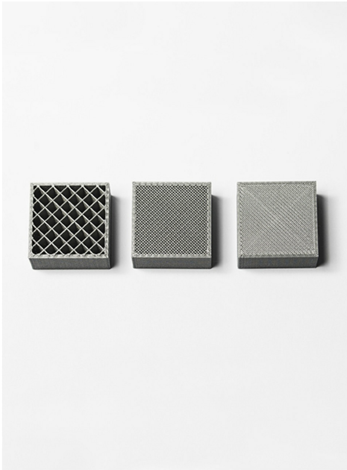
Figure 11.13– Infill percentage variations ranging from 20% (left), 50% (center) and 75% (right)
