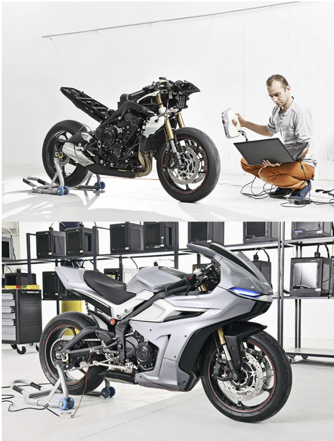
Figure 18.4–A hand held laser scanner being used to generate a 3D model of a motorcycle frame (top). Using the 3D scan data, the body panels of the motorcycle were designed and then 3D printed on a Zortrax FFF printer (bottom). Images courtesy of Zortrax
