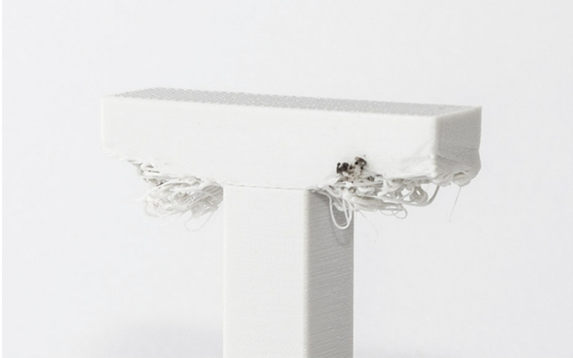
Figure 11.4– The letter T fails when printed on an FFF printer without any support structures
