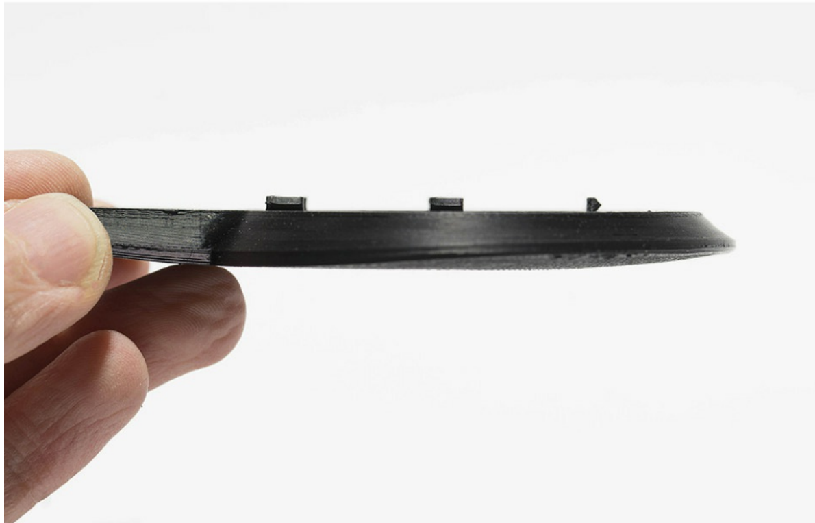
Figure 2.5 – A warped FFF part printed in ABS
