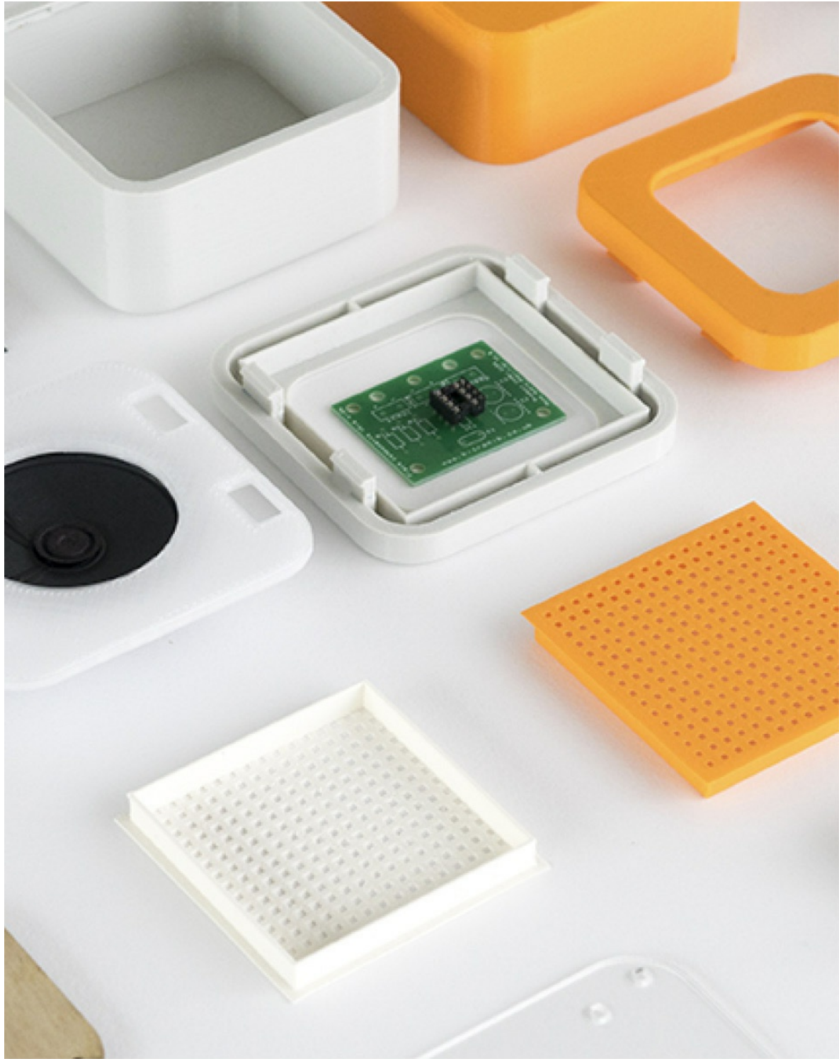
Figure 2.19 – A disassembled portable speaker with plastic parts printed on a desktop FFF printer
