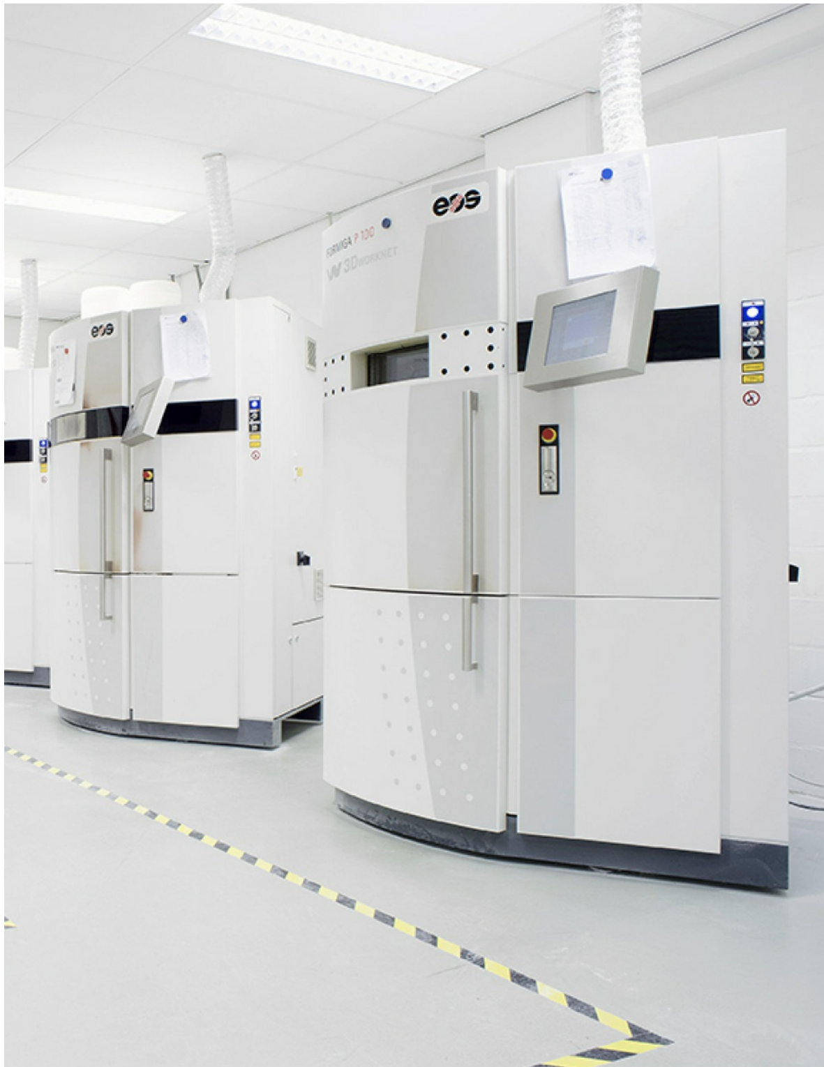
Figure 4.4– A group of SLS printers allow for high output manufacturing
