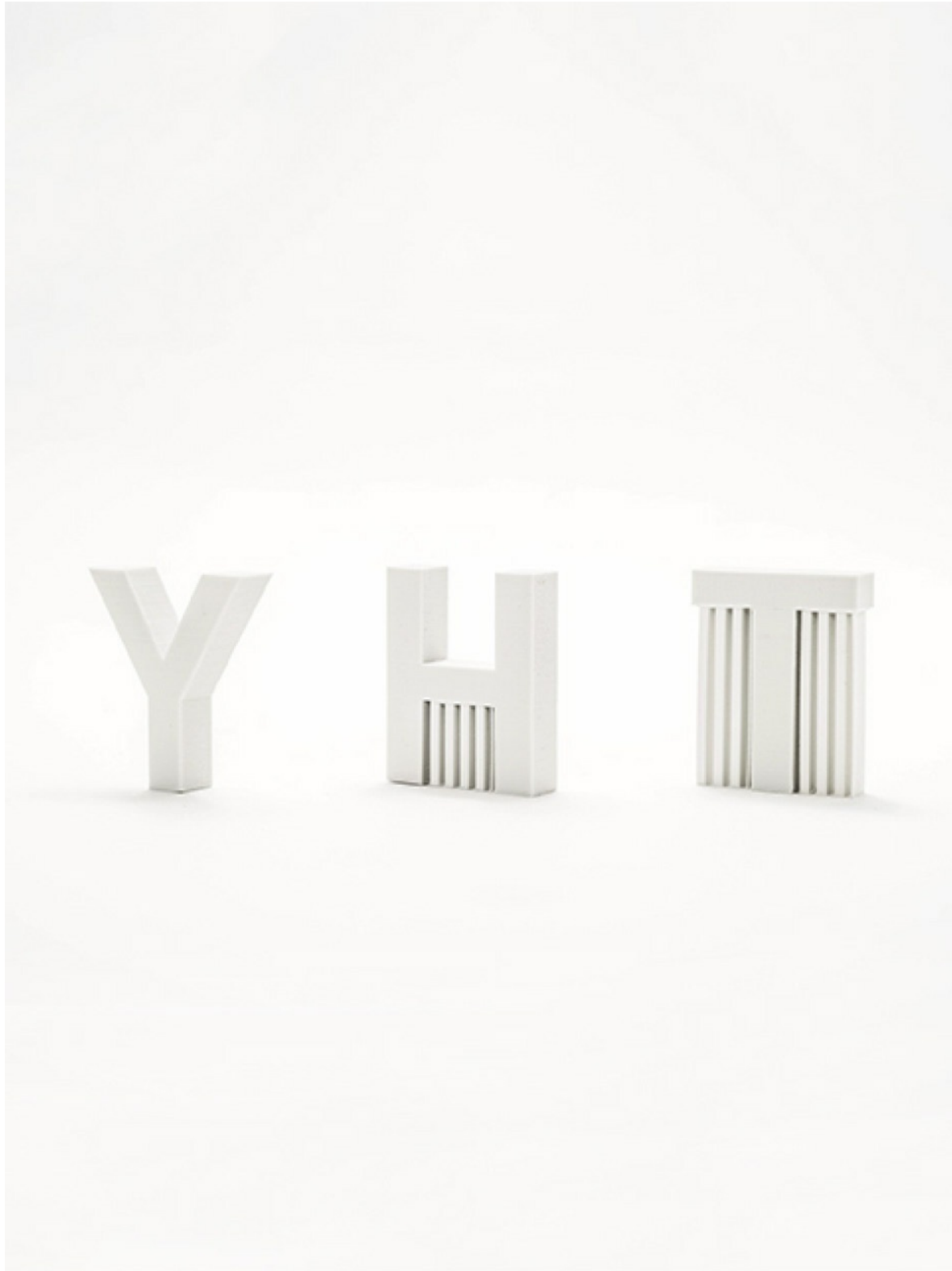
Figure 11.3– Y, H, and T printed on an FFF printer showcasing support requirements
