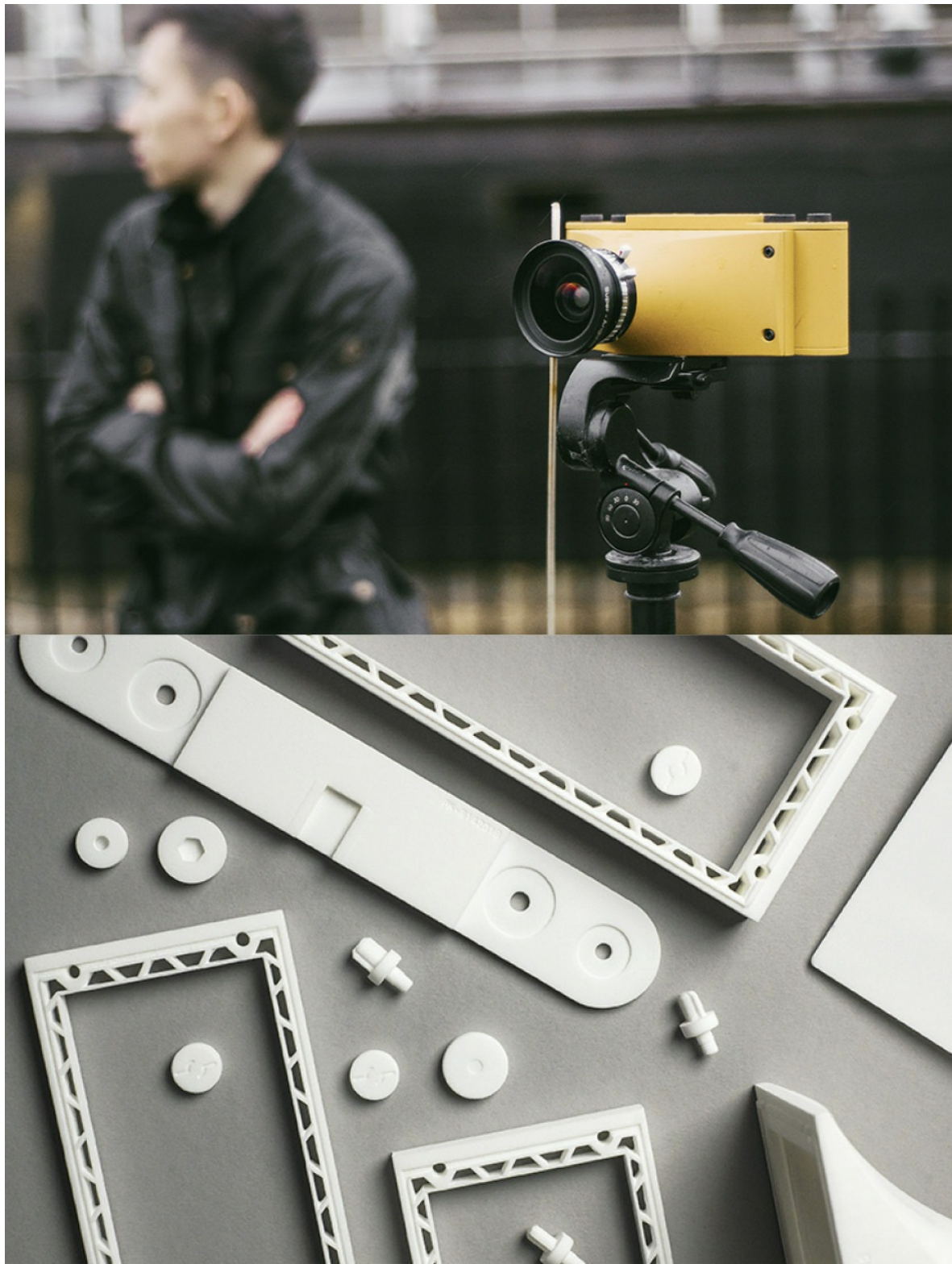
Figure 21.2–The finished camera with the yellow housing 3D printed with SLS nylon (top). The SLS nylon parts of the camera before painting (bottom)
