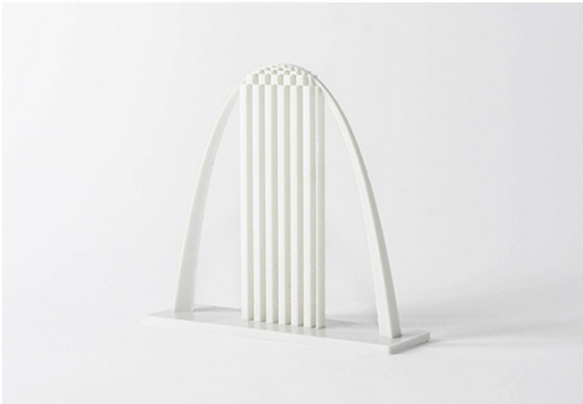
Figure 11.5– This arch illustrates how support is only required at certain areas on curved surfaces
