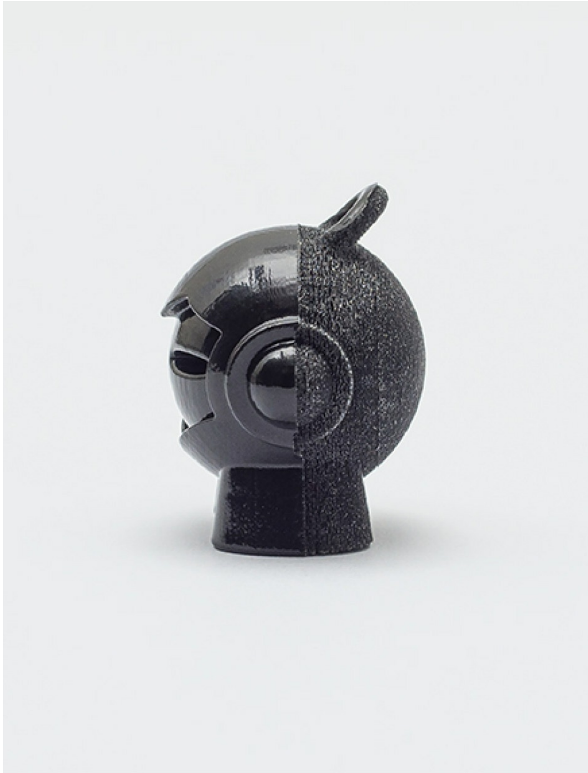
Figure 5.6–A Material Jetted part, TangoBlack (rubber-like), printed in half glossy, half matte, showing the difference in surface finish
