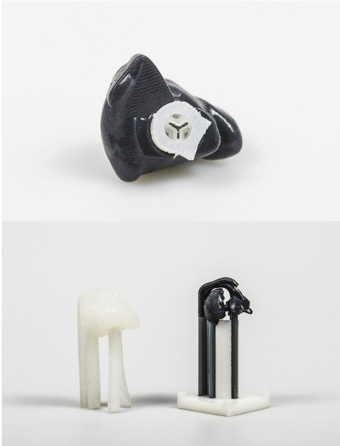
Figure 22.1–The final 3D printed heart used in the manikin showing the silicon molded working valve (top). The outer mold (white) and inner core (black) of the mold shown here were used to produce a hollow functional silicon model of a lung (left). The inner core needed to be made of a flexible material to aid in removal after the silicon had set (bottom)
