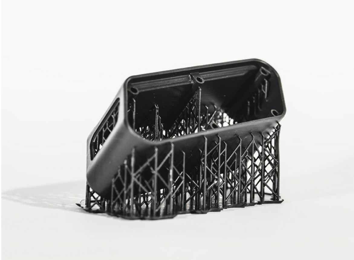
Figure 12.1 – An SLA printed enclosure with support material still attached
