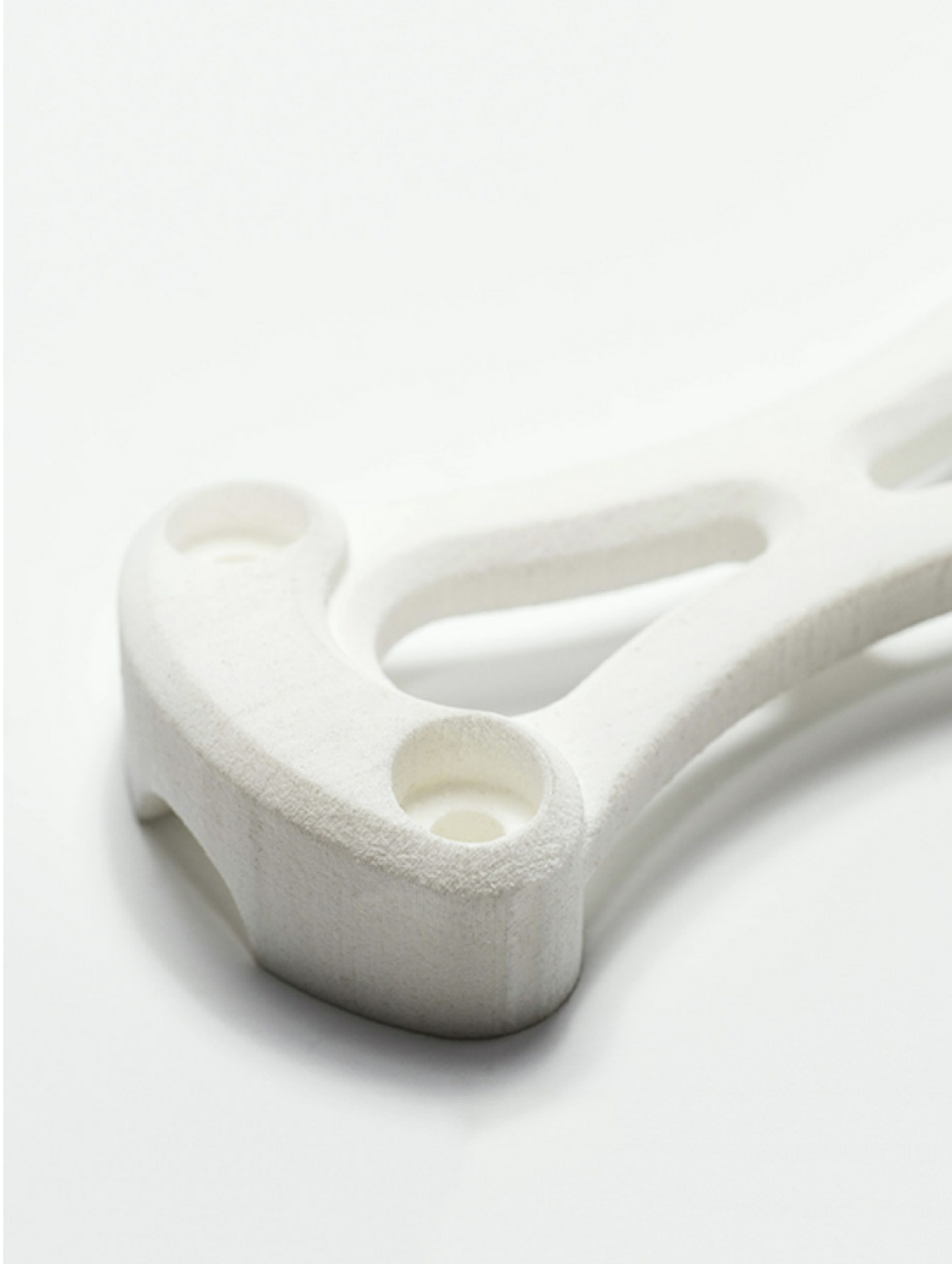
Figure 4.5 – SLS printed bracket with its characteristic white Nylon appearance. A slightly grainy surface is visible upon close inspection
