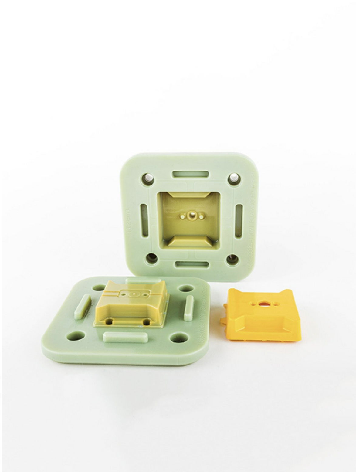
Figure 5.9—A low run injection mold printed from Digital ABS, used to produce a batch of sensor housings. Image courtesy of Promolding
