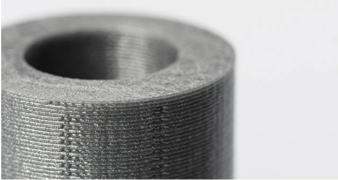
Figure 2.8 – The layer lines of an FFF part are generally visible
