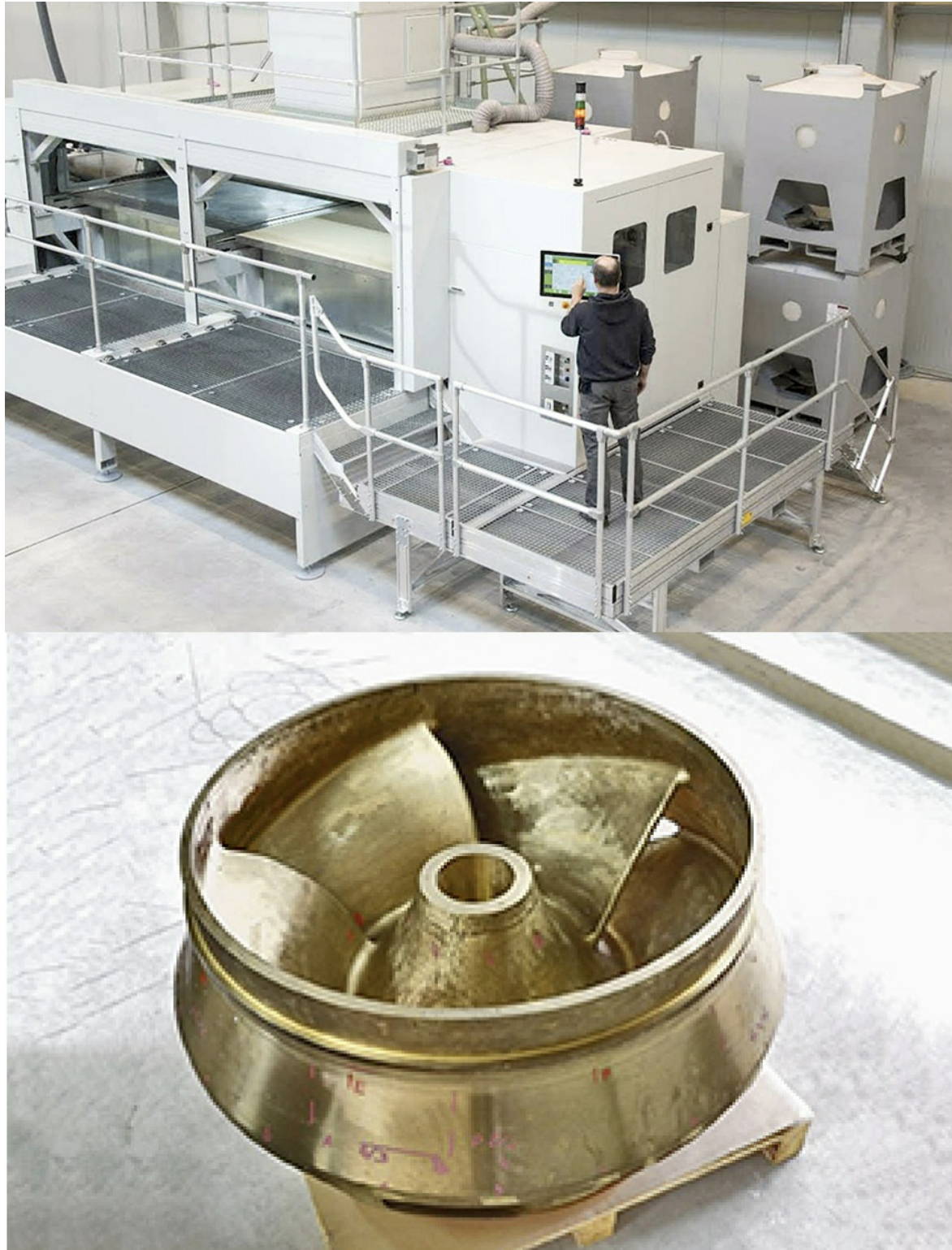
Figure 23.2 – The ExOne Exerial is used for the production of sand casting molds and has a build volume of 2200 x 1200 x 600 mm making it one of the biggest 3D printers (top). The final vertical pump impeller cast from bronze using a modular sand cast printed by Binder Jetting (bottom). Images courtesy of ExOne
