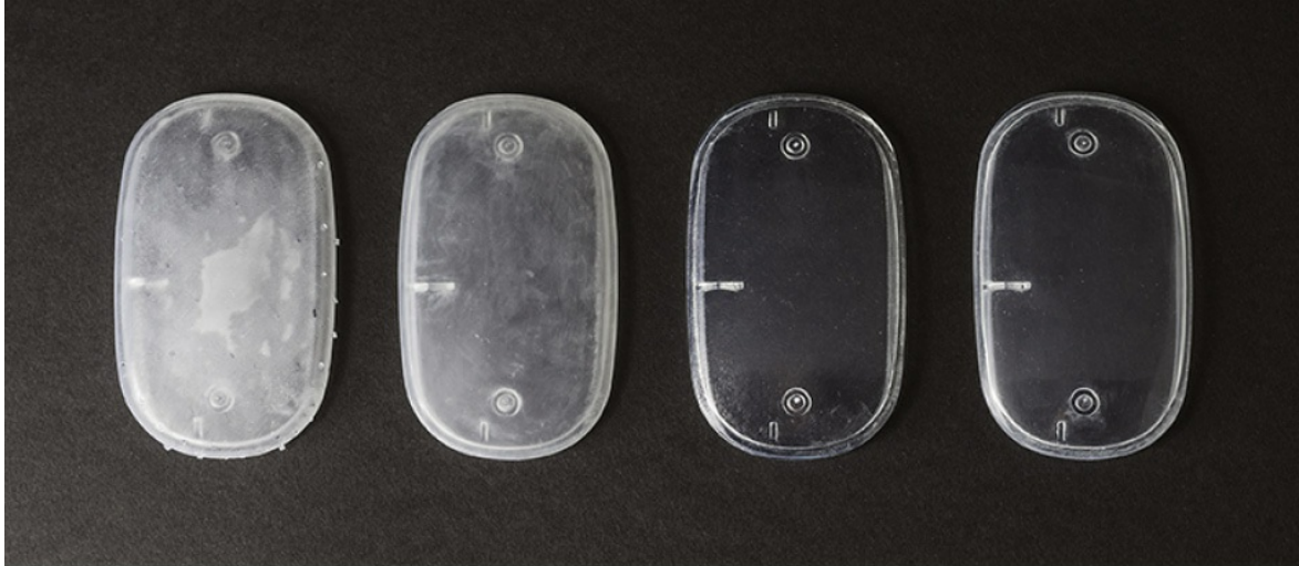
Figure 3.11 – Transparent resin electronic housing cover with a range of post processing finishes. From left to right; basic support removal, wet sanding, UV protective acrylic lacquer and polished
