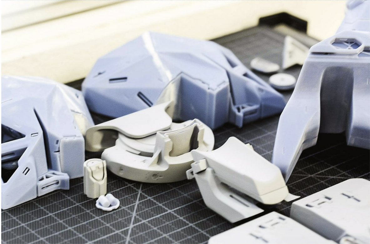
Figure 22.3–A piece of the Ultraborg model showing the smooth surface and detail produced by Material Jetting (top). Parts during post processing (bottom). Images courtesy of Factor 31
