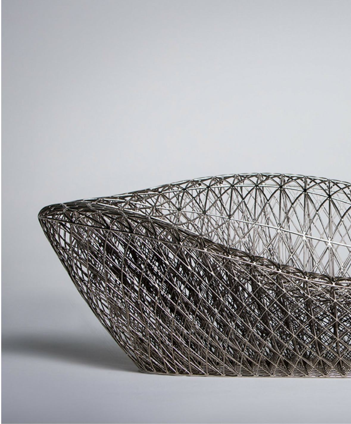
Figure 3.12 – Industrial sized Vat Polymerization printers can have some of the largest build volumes of all 3D printing technologies. This was utilized when manufacturing Sofa So Good, a full sized lounge printed on an industrial SLA printer and then metal coated in high polish copper and chrome (making the couch functional). The lounge measures 1500 x 750 x 550mm, yet weighs only 2.5 kilograms and was created using just 2.5 liters of resin. Sofa So Good was 3D printed from 6000 layers, each 100 microns thick, in a single print. The unique diamond geometry creates a super strong structure that can support a person weighing up to 100 kilograms. Image courtesy of Janne Kyttanen
