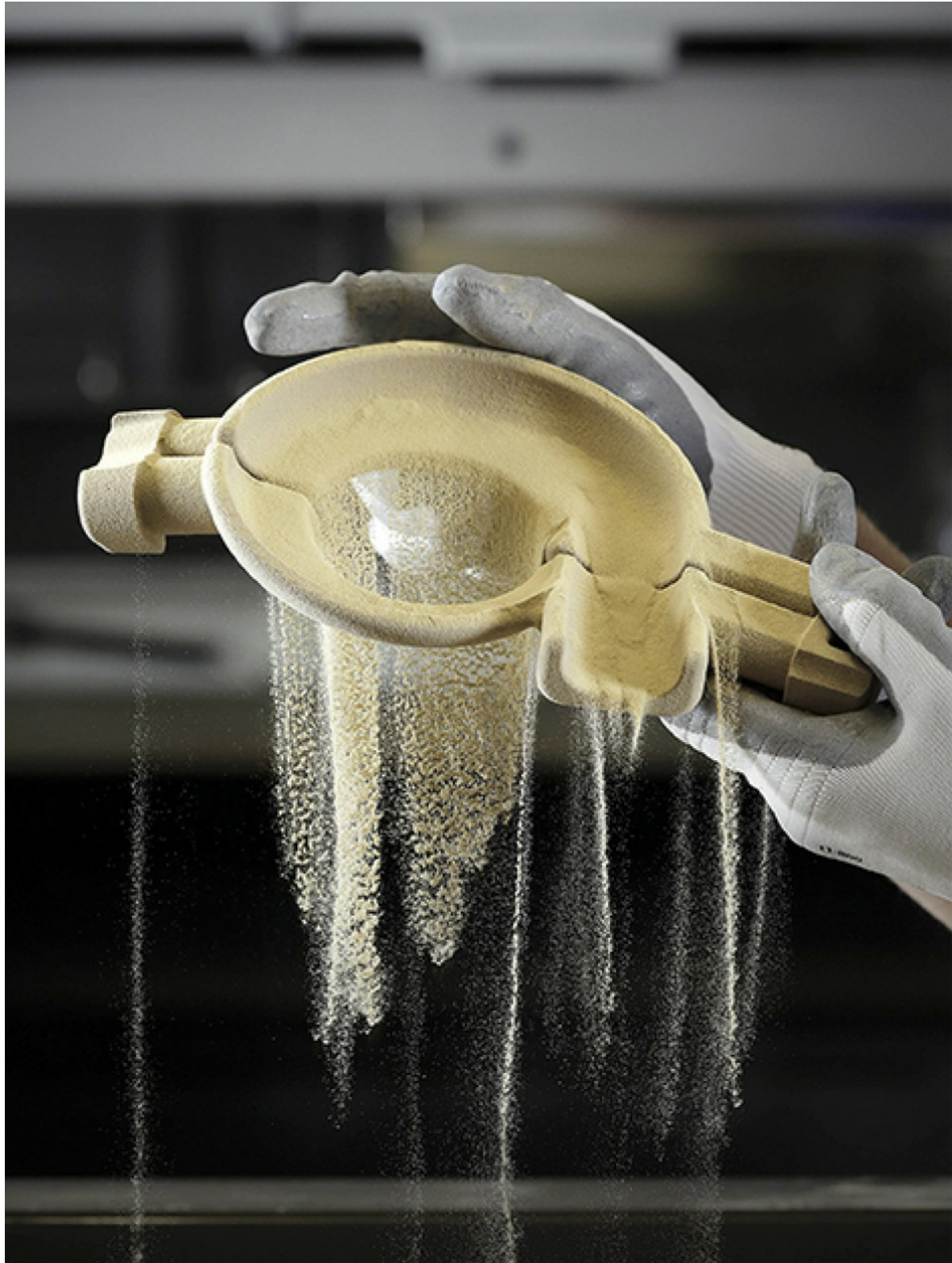
Figure 6.5 – Loose powder being removed from a part produced via Binder Jetting. Image courtesy of ExOne
