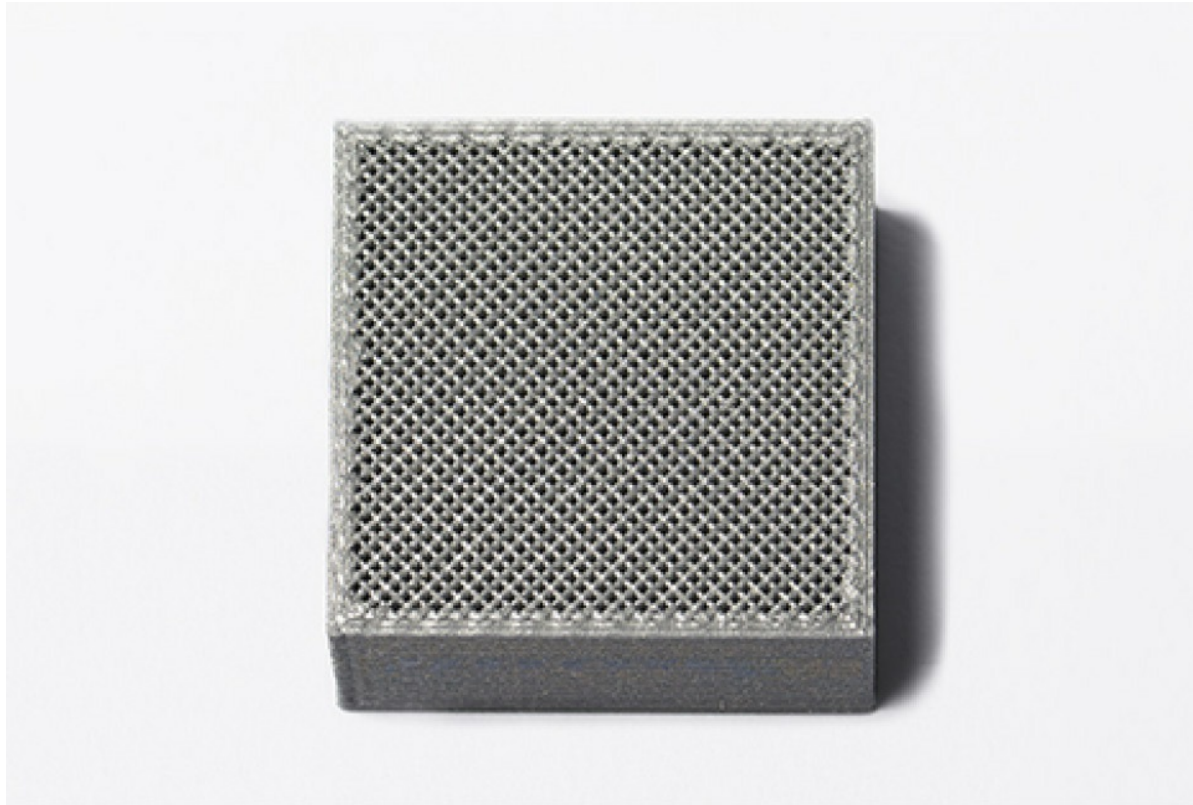
Figure 2.11 – The internal infill geometry of an FFF print
