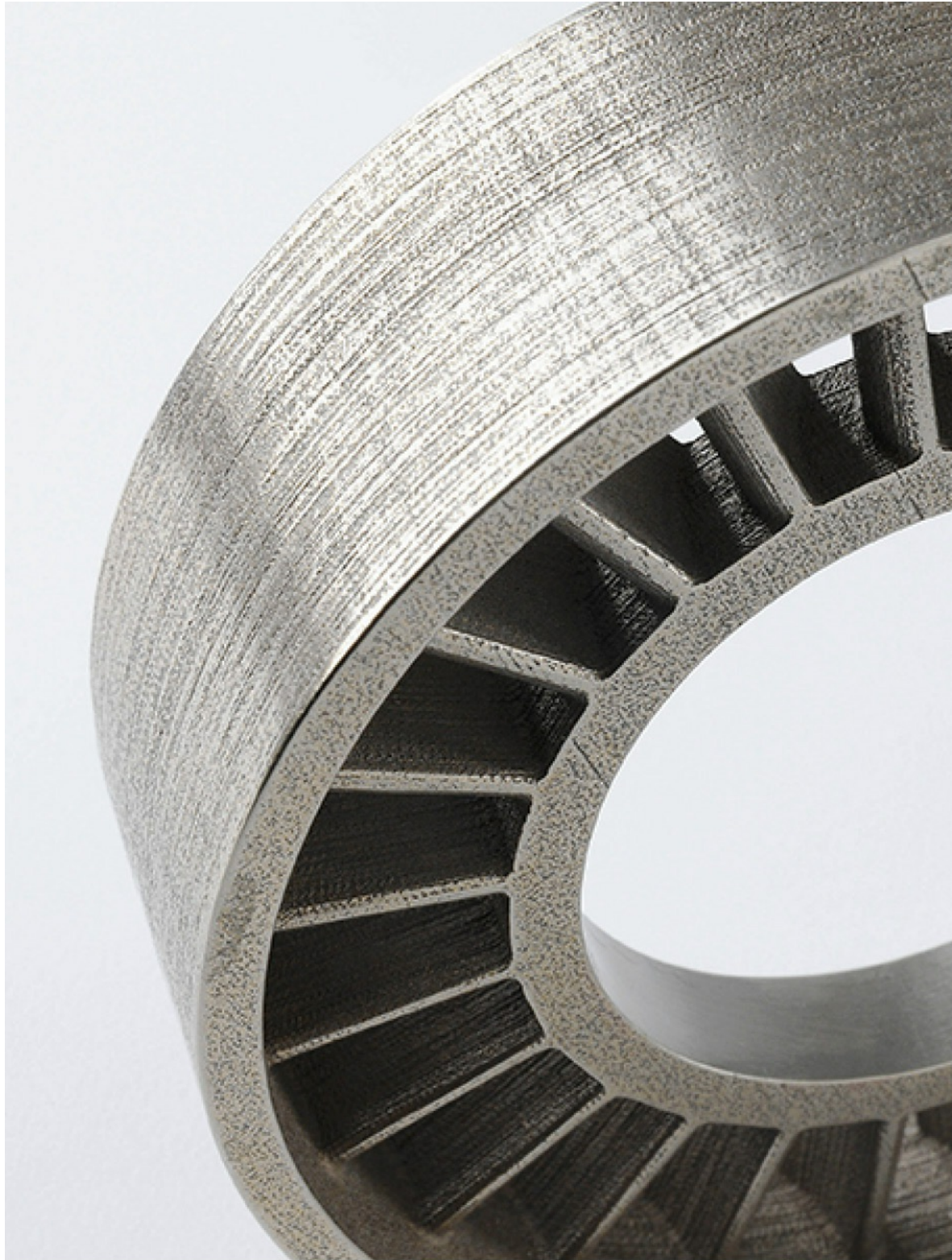
Figure 6.7 – An oil and gas stator printed from stainless steel and infiltrated with bronze. Image courtesy of ExOne
