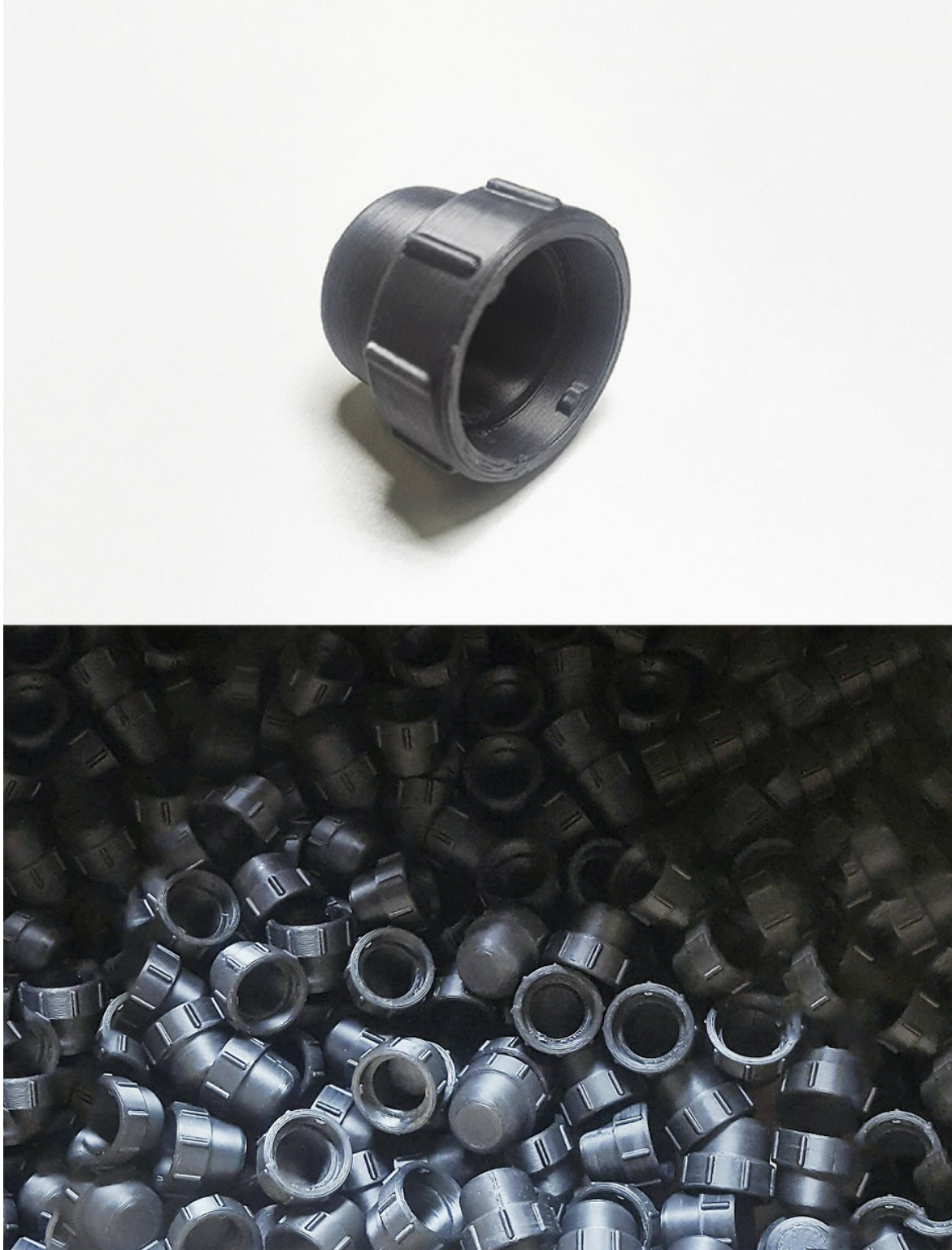
Figure 19.6 – The final caps printed from ASA via FFF (top). Industrial FFF allows for cost-effective batch manufacturing at low to mid-volume production (bottom). Images courtesy of Peak Additive
