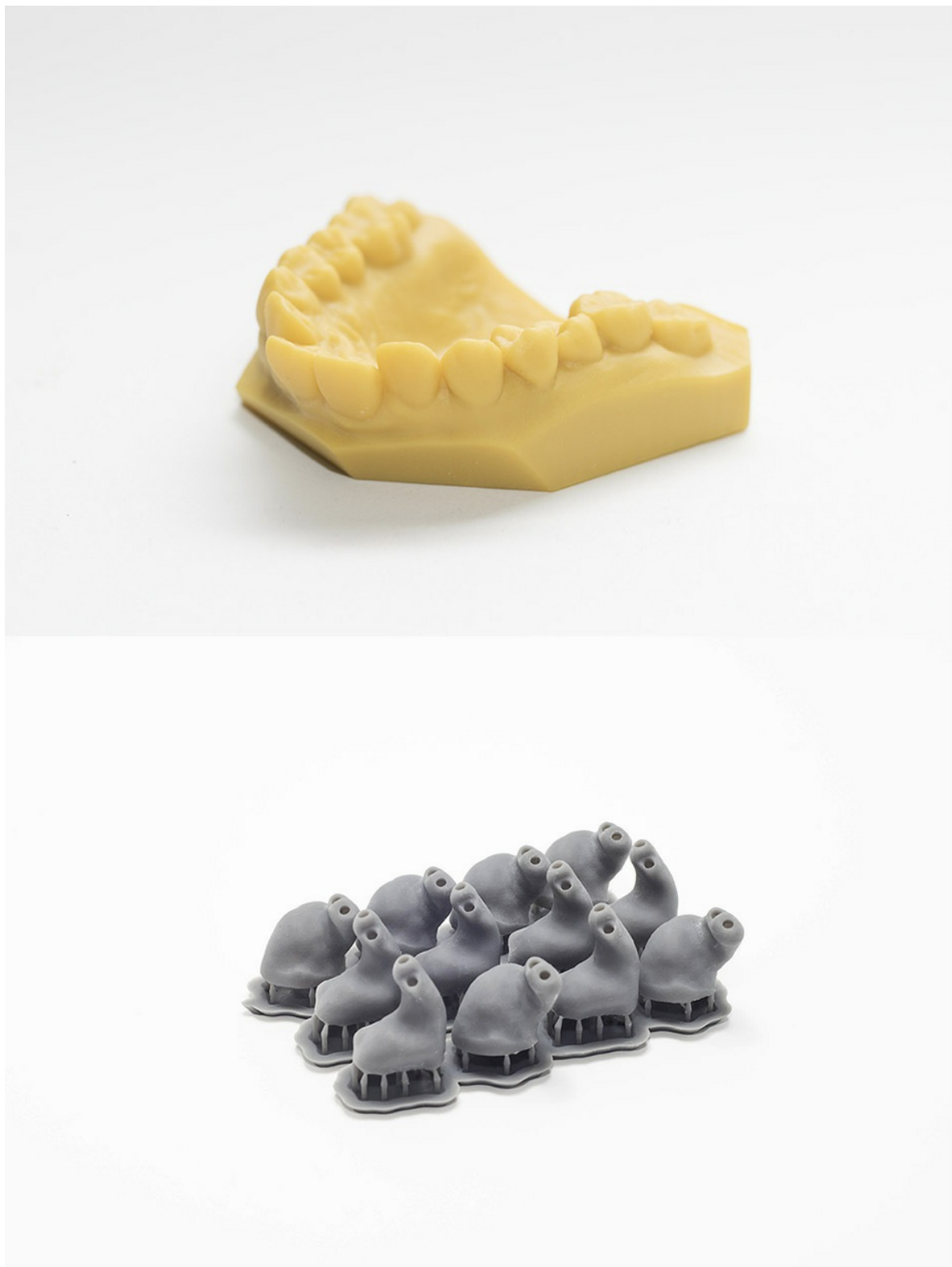
Figure 3.13 – A dental model printed from a 3D scan of a patient's mouth (top). A batch of custom hearing aids printed on the Formlabs Form 2 printer (bottom)
