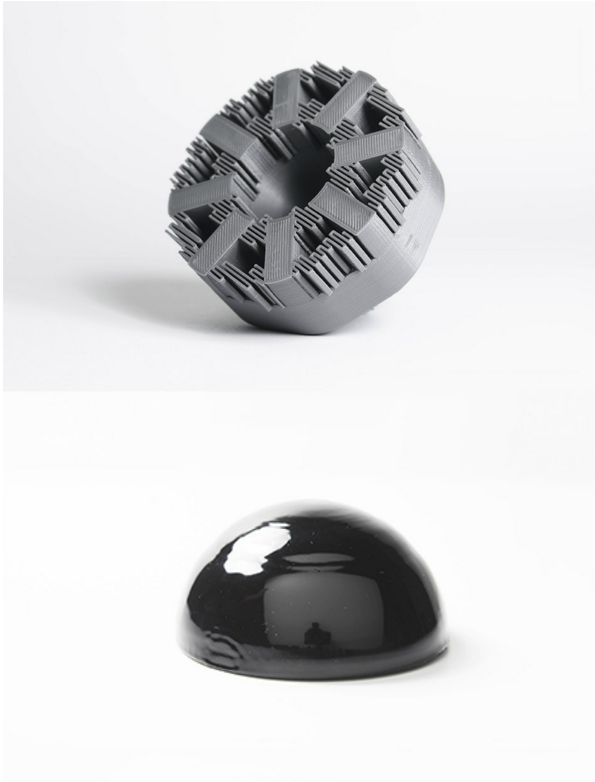
Figure 2.14– FFF part with support still attached illustrating the lattice geometry of support structures (top). A vapor polished ABS hemisphere (bottom)
