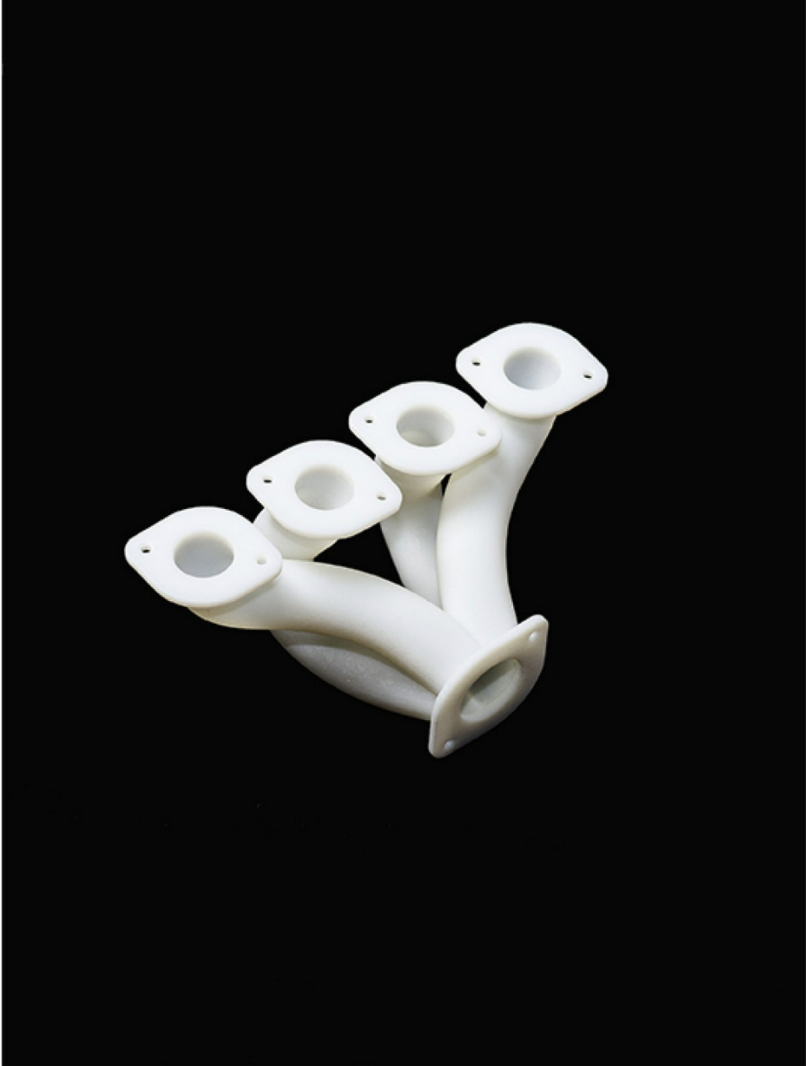
Figure 4.8 – Functional SLS ducting used in an automotive application
