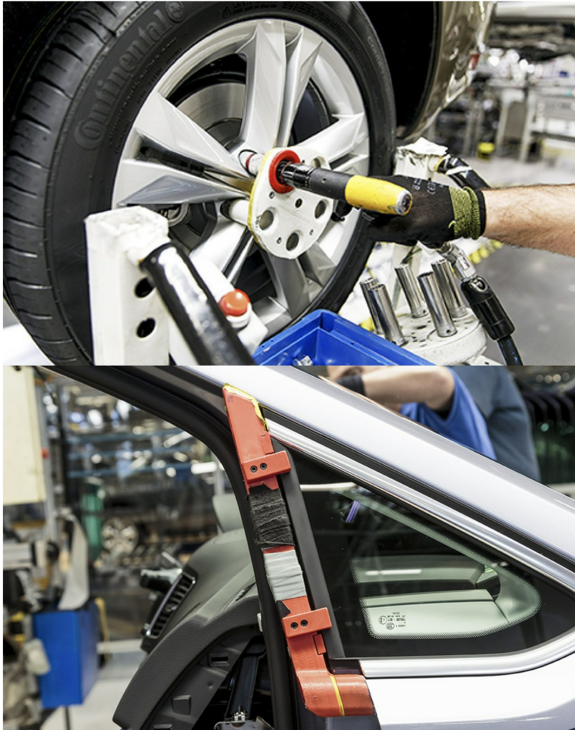
Figure 19.2– This 3D printed wheel protection jig previously sourced via traditional manufacturing for €800, now 3D printed inhouse at €21 per part. Tool development time shrunk from 56 to 10 days (top). This window gauge originally cost €180 per part to get made via traditional manufacturing externally. It is now 3D printed at just €35. Development time went from 8 to 6 days (bottom). Images courtesy of Volkswagen Autoeuropa and Ultimaker
