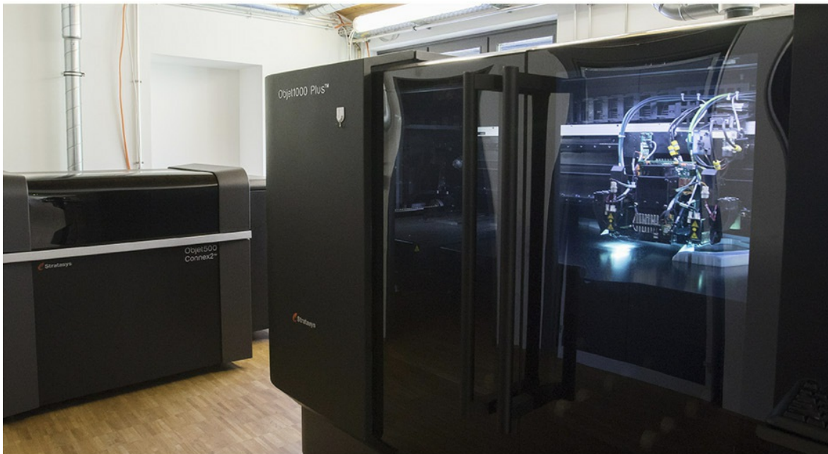
Figure 5.4 – The Stratasys Objet100 Plus printer illustrating the size of some Material Jetting printers
