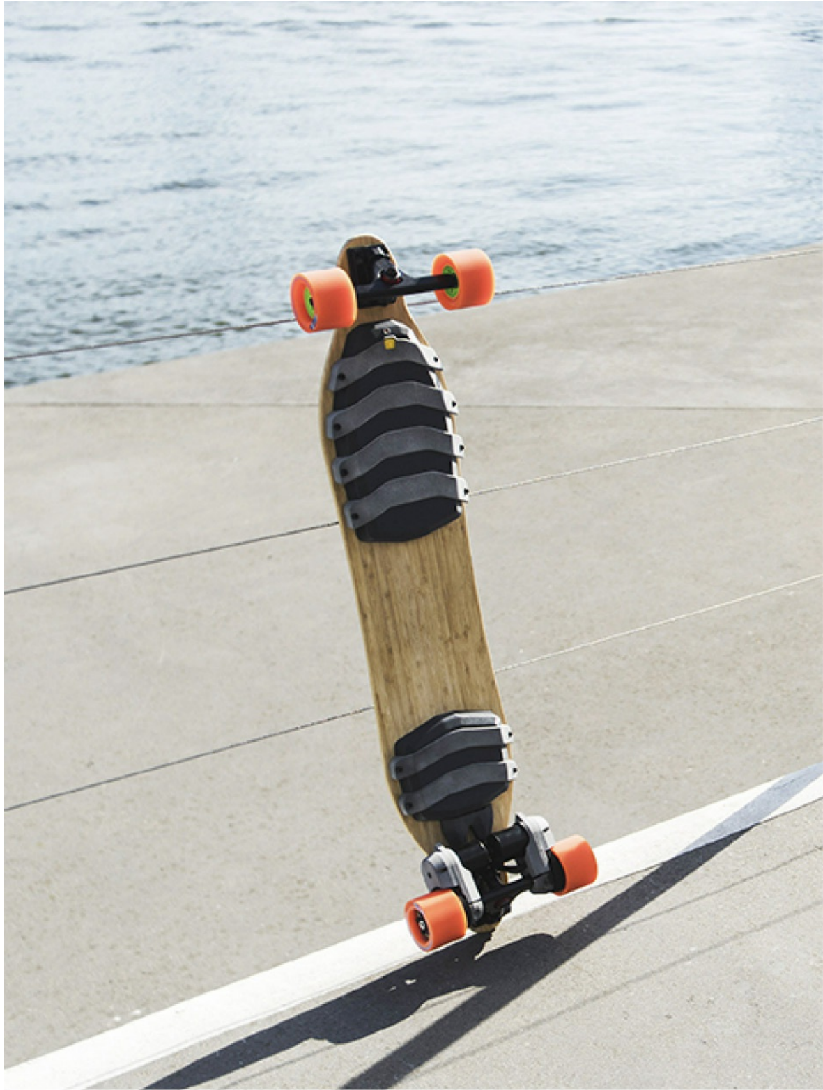
Figure 4.9 – Brackets and motor housings on an electric skateboard printed via the HP 3D4200 printer
