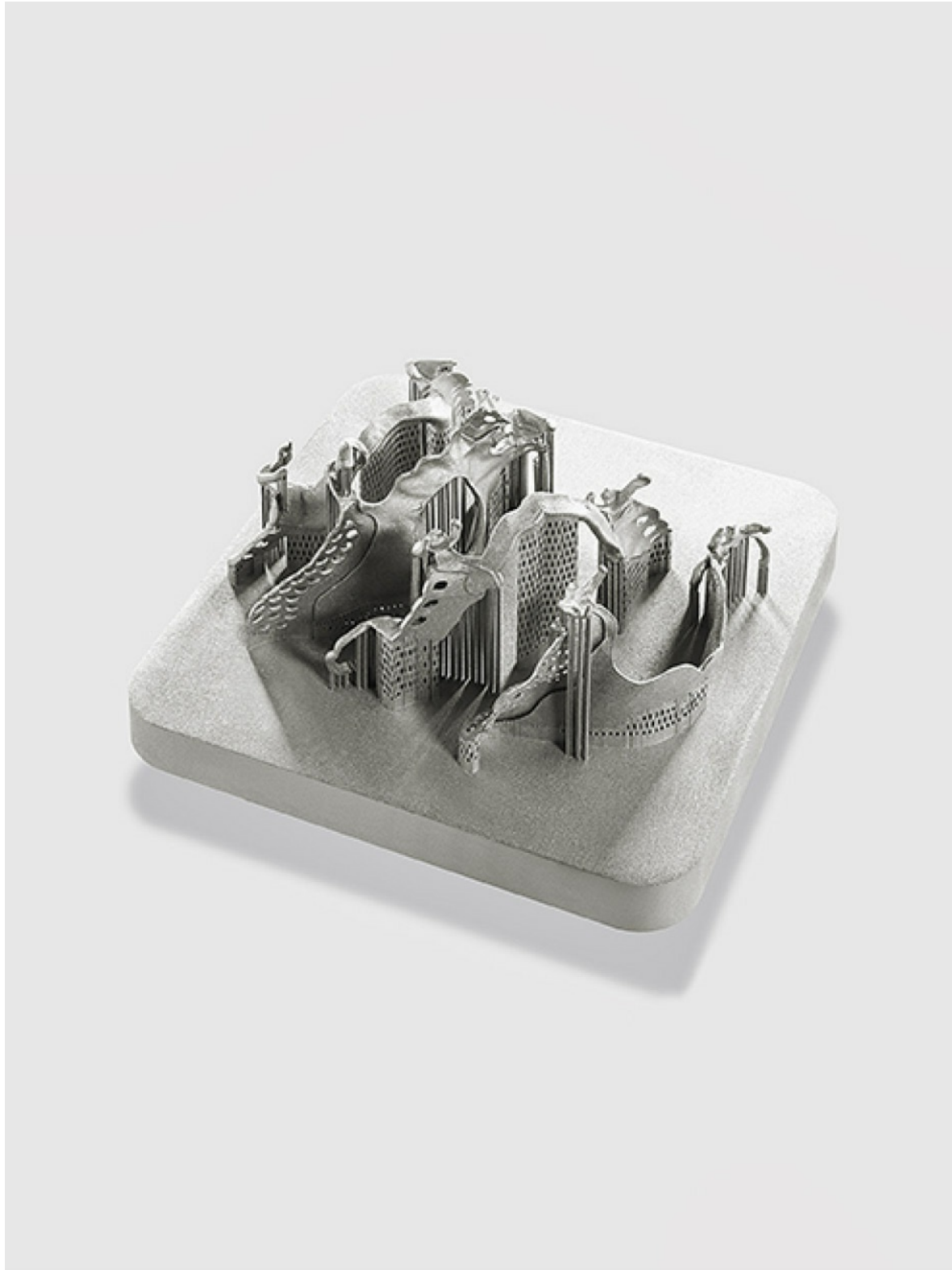
Figure 16.1 – Dentures printed for use in the dental industry. The parts shown here are still attached to the build plate and with support structures still connected. This image gives an insight into the amount of support a build requires to successfully print. Image courtesy of Concept Laser GmbH
