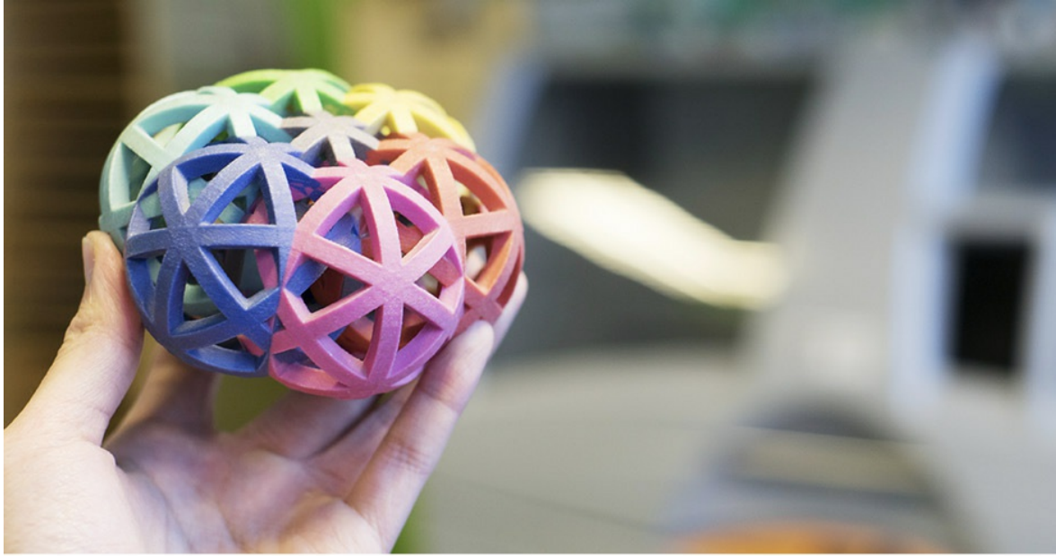
Figure 6.3–A full color print produced using Binder Jetting sandstone
