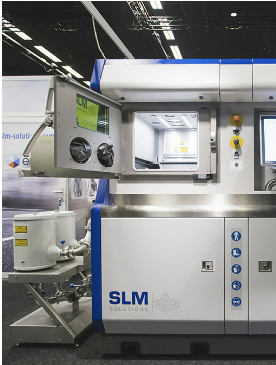
Figure 16.5 – An SLM machine showing the build chamber (280 x 280 x 365 mm) in the center relative to the size of the machine
