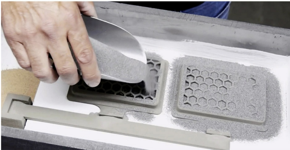
Figure 6.4– Stainless steel parts being covered with sand before infiltration. The bronze infiltrant is shown on the left. Image courtesy of ExOne
