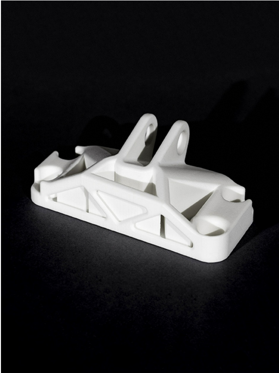
Figure 13.7– A hollow, functional bracket printed using SLS nylon showing slots for powder removal
