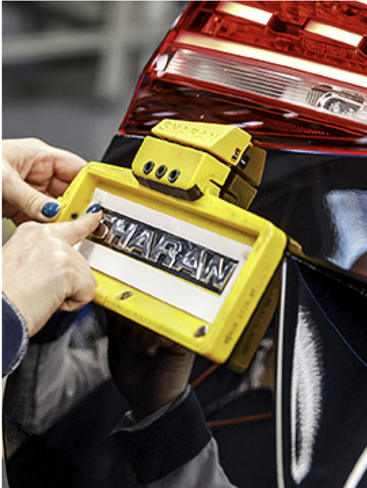
Figure 19.3—This liftgate badge took 35 days in development time when produced via traditional manufacturing externally and used to cost €400. With 3D printing, the project was completed in 4 days and the cost of the part reduced by more than 90%. Image courtesy of Volkswagen Autoeuropa and Ultimaker
