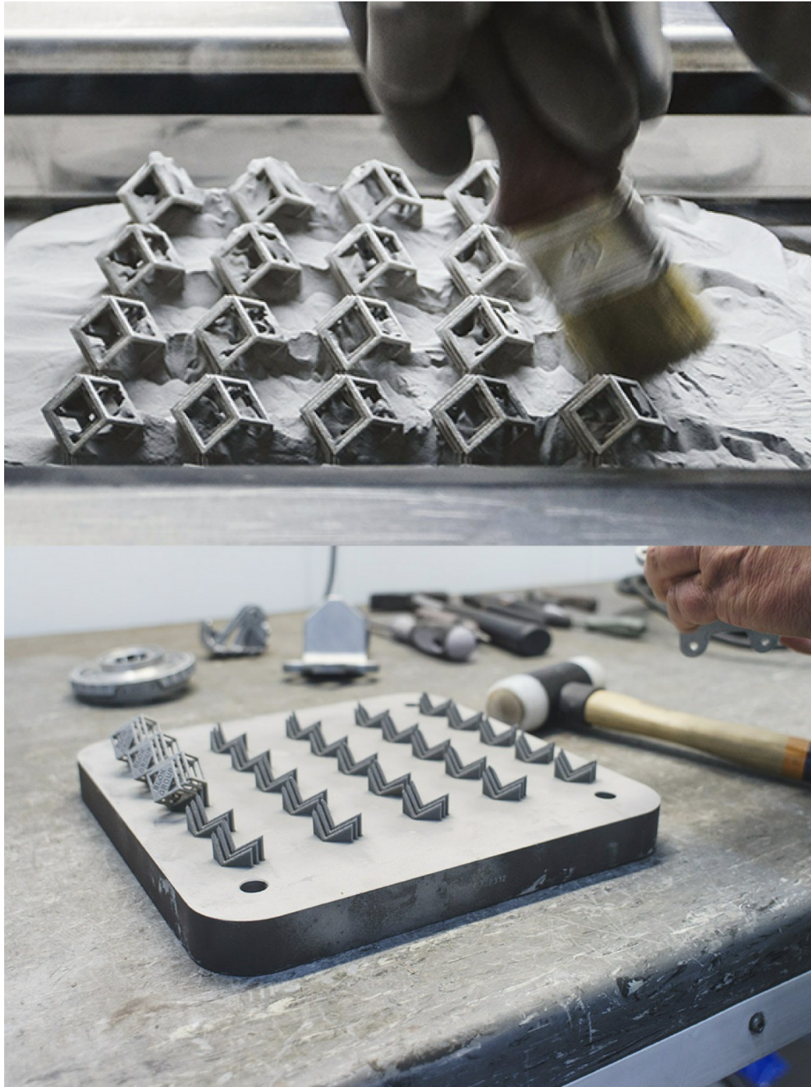
Figure 16.3– Powder being removed from metal parts produced by the SLM printing process (top). SLM printed parts being removed from the build plate (bottom)
