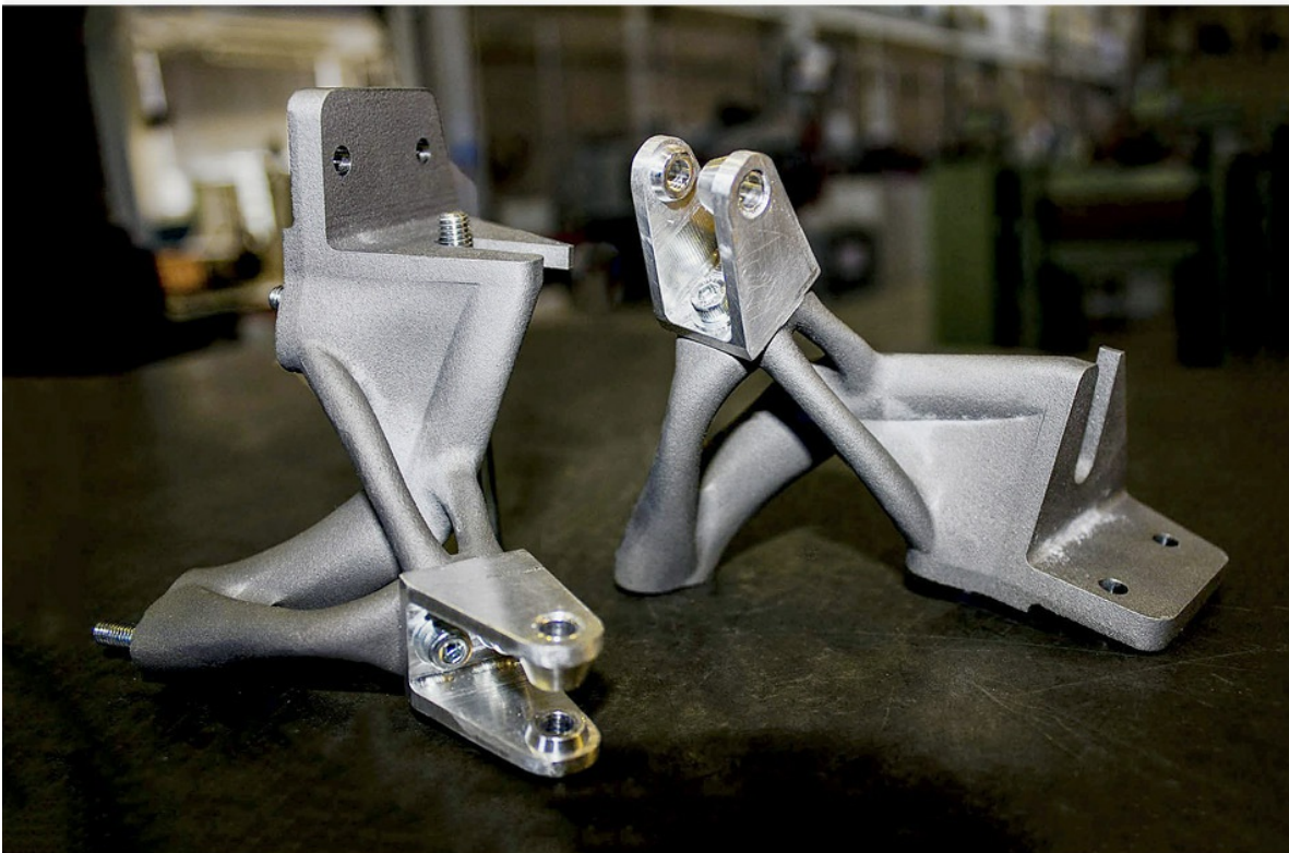
Figure 24.2 – Output geometry from topology optimization process, on the left, and the final bracket design, shown on the right (top). The final suspension brackets printed from titanium via the SLM process. The bracket was also machined after printing (bottom). Images courtesy of TU Delft Formula Student Team
