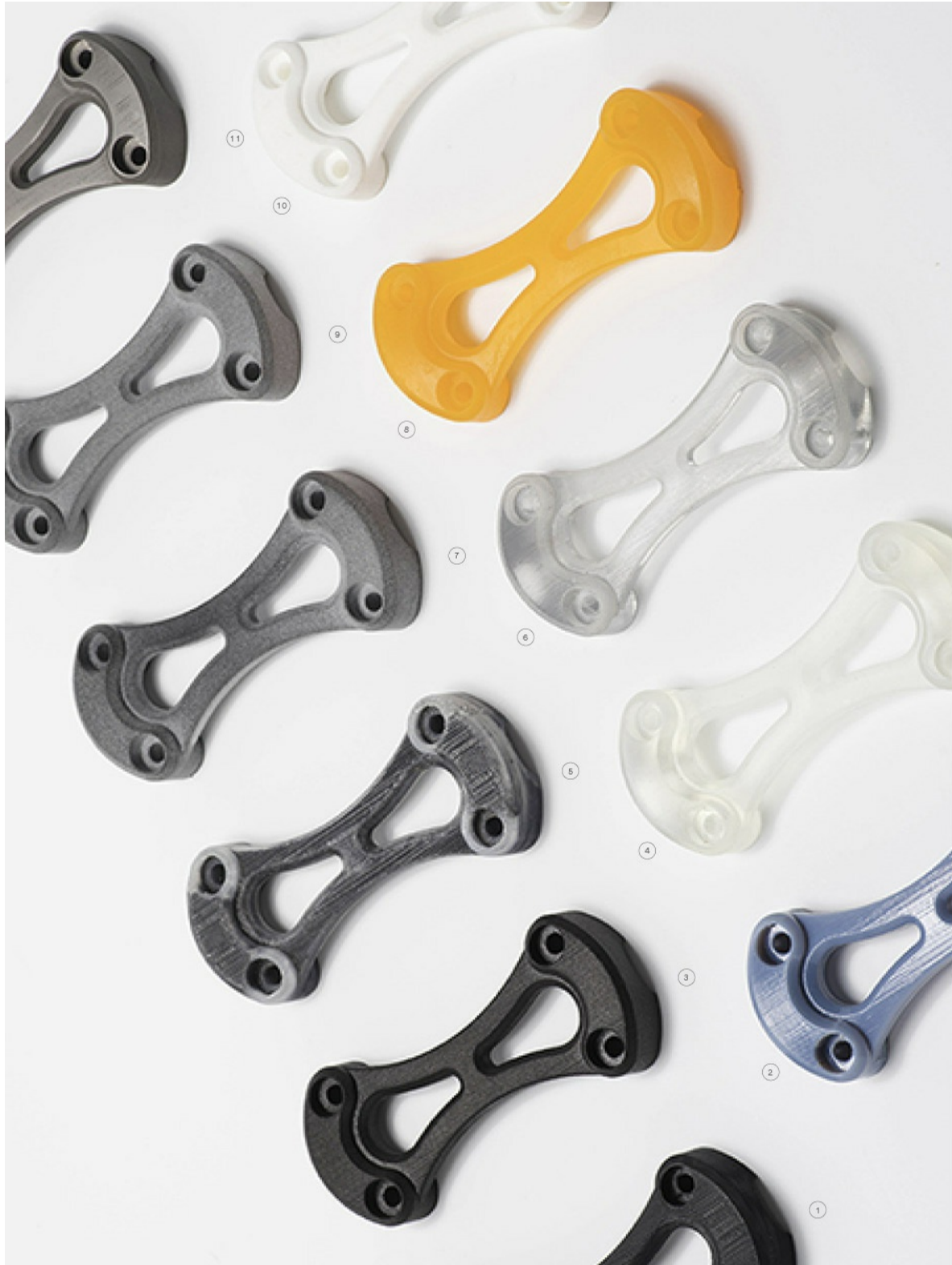
Figure 1.3–A range of different 3D printed materials showing: 1. ABS (FFF), 2. rigid opaque resin (Material Jetting), 3. graphite-reinforced nylon (SLS), 4. transparent resin (SLA), 5. carbon-reinforced nylon (CFF), 6. ultra clear resin (Material Jetting), 7. HP nylon (Multi Jet Fusion), 8. castable resin (DLP), 9. grey PA12 nylon (SLS), 10. white PA12 nylon (SLS), 11. tool steel (DMLS)
