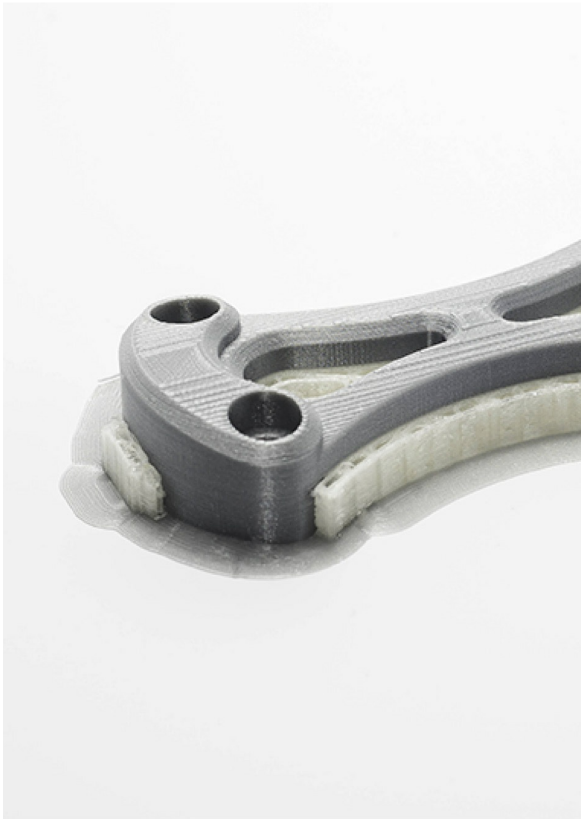
Figure 2.10 – An FFF bracket printed in PLA (grey) showcasing dissolvable PVA support (white)
