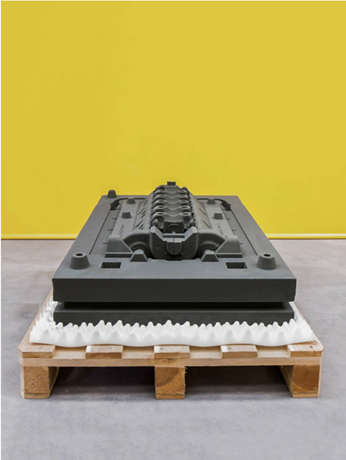
Figure 6.6–A multi-part sand casting assembly used to cast an engine block. Image courtesy of ExOne
