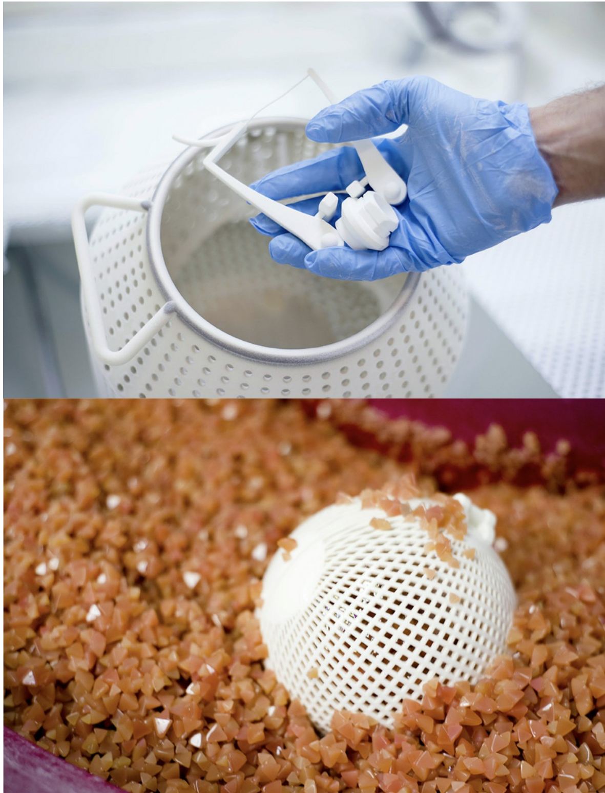
Figure 4.6 – SLS post processing showing; powder removal (top), medium polishing (bottom)
