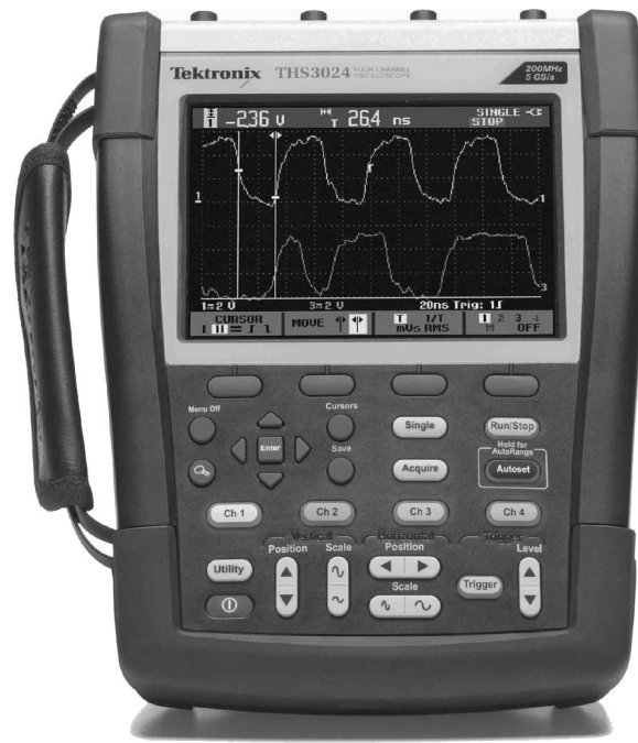
FIGURE 16-3 Tektronix digital oscilloscope with cursor to define portion of waveform to be measured. (Courtesy of Tektronix.)
